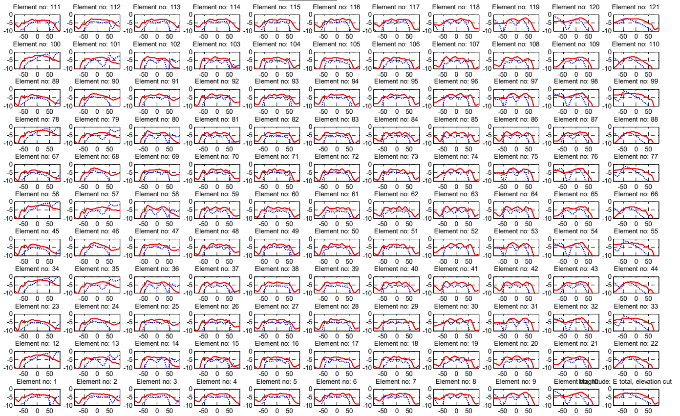
Figure 11.12: 11x11 RDRA array in a triangular grid: E-plane embedded patterns
