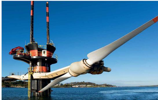
**Figure 2.14** SeaGen-S turbines [13] [©Marine Current Turbines-A Siemens business].
