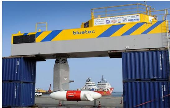
**Figure 2.16** Tocardo T1 turbine mounted under floating BlueTEC platform. Image source [39].
