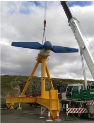
**Figure 2.3** Horizontal axis tidal stream turbine: NOVA M100 [©Nova Innovation] [6] .
