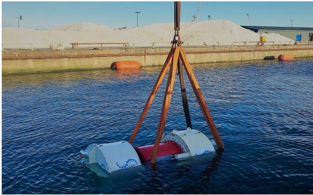
**Figure 6.16** In-sea testing of TiPA PTO at Babcock's Rosyth site.
