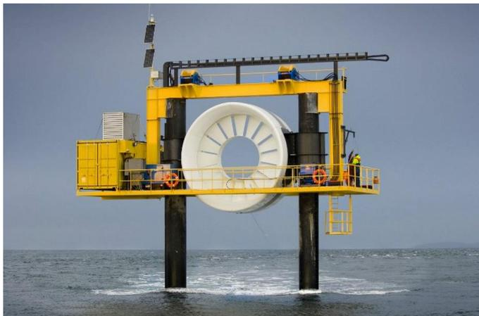
**Figure 2.8** DCNS OpenHydro's rim-driven generator, reproduced from [27]; (Credit: Mike Brookes-Roper).
