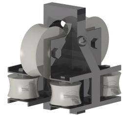
Figure 7.25: Wheel system for lateral movements on the rail.
