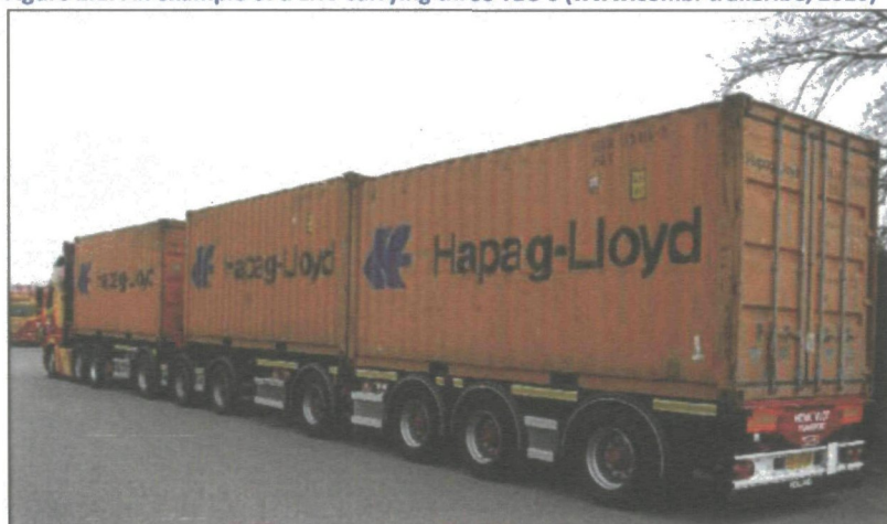
Figure 2.1: An example of a LHV carrying three TEU's ( www.combi-trailer.be , 2010)
