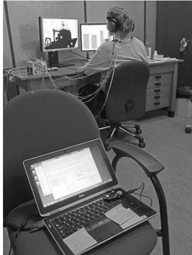
Figure 7.6 Experimental setup. In the foreground trainer part of COPE-FB system with Zephyr HxM heart on keyboard. In the background a participant views the ship simulation on the left and the trainee part of COPE-FB system on the right.
