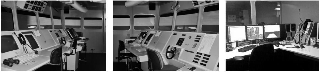
Figure 4.2. Bridge simulator based on the “Van Tromp” ship, seen from 2 angles and the trainer control room.
