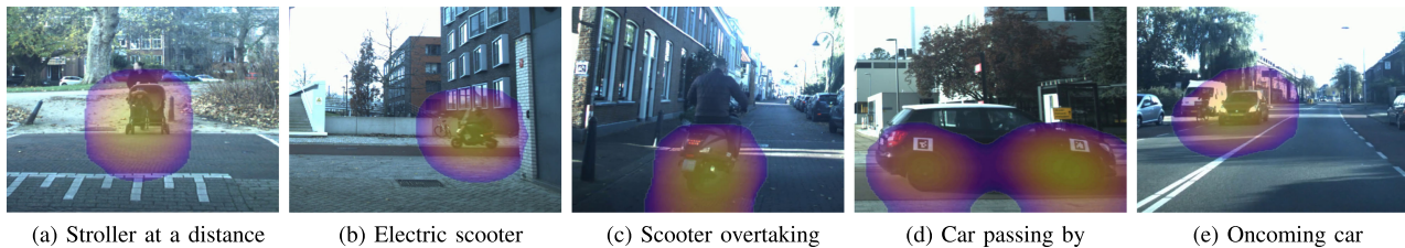
Fig. 4. Qualitative examples of 2D Direction-of-Arrival estimation overlaid on the camera image (zoomed). (a): Stroller wheels are picked up even at a distance. (b), (c): Both conventional and more quiet electric scooters are detected. (b): The loudest sound of a passing vehicle is typically the road contact of the individual tires. (e): Even when the ego-vehicle drives at \sim 30 km/h, oncoming moving vehicles are still registered as salient sound sources.
