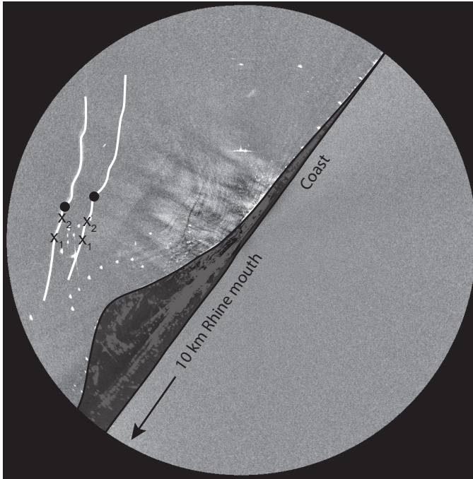
Figure 3.11: Front tracking system. Frontal speed is estimated by comparing radar images at two different times (white lines). Black crosses are used to estimate the frontal propagation speed and the black dots indicate the alongshore movement. Image is of September 17th 2014, 09:42 - 09:57 (day 260).
