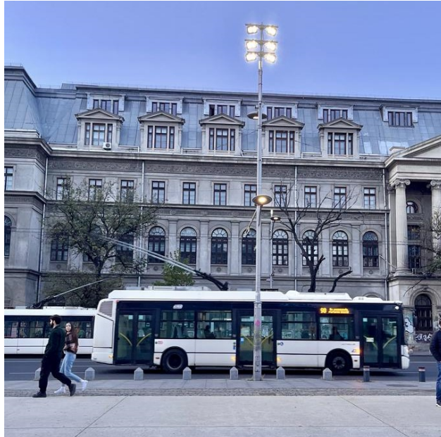
Figure 1.1: A trolleybus and its pantograph in Bucharest, Romania. Here, the overhead cables can be seen connected to the public lighting poles (Photo by author).
