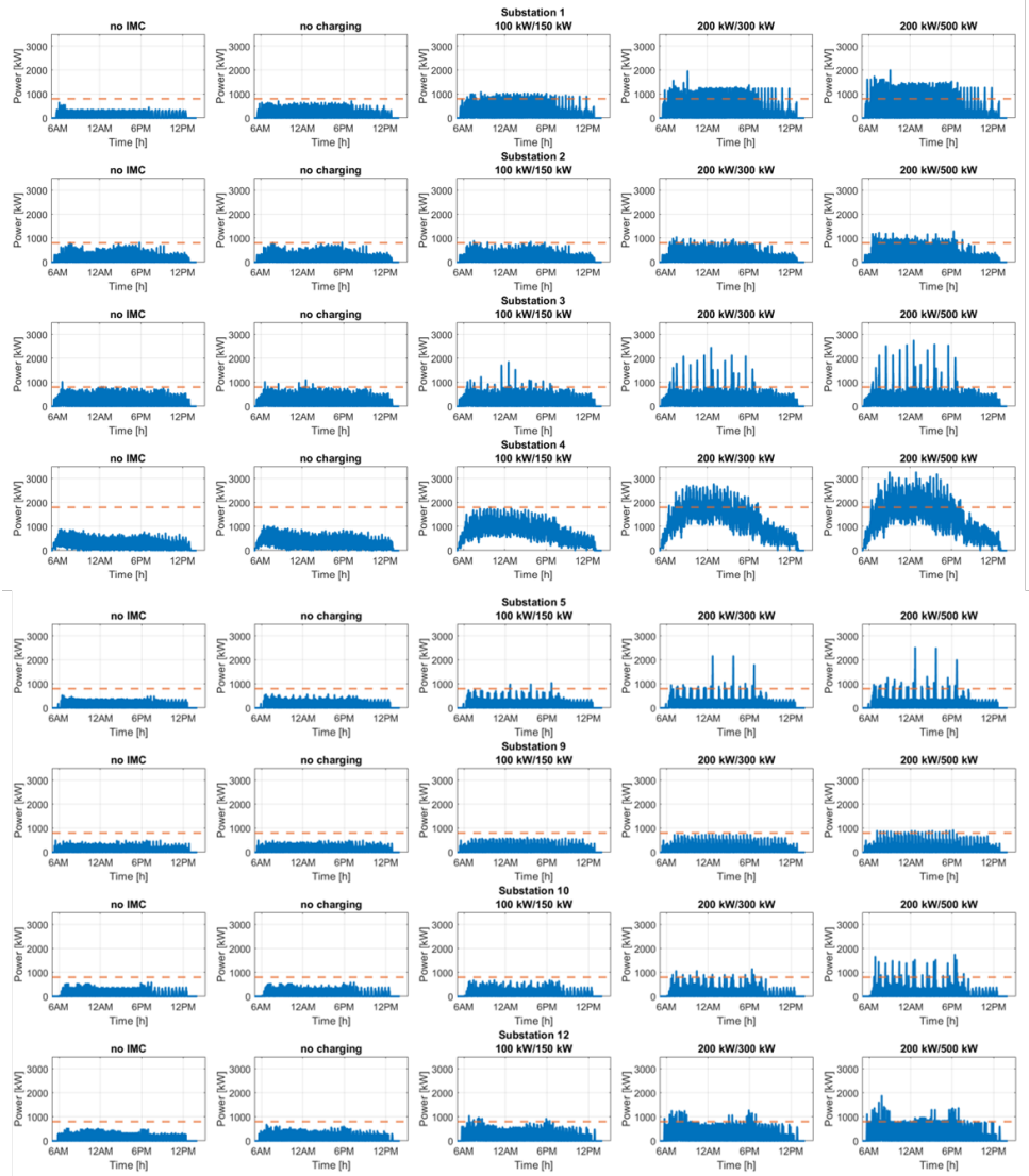
Figure 11.8: Closer look at the substation power demand on a Regular Weekday schedule for five IMC battery charging schemes.
