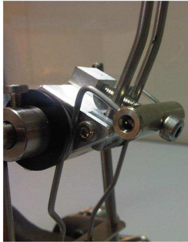
Figure 1: Pretension system of the upper spring. The torsion springs pokes run through a tube of which the position can be determined by adjusting the screw in the upper pivot.
