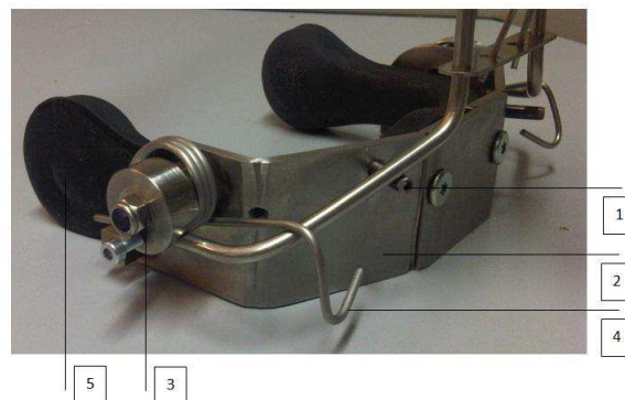
Figure 3: Photo of the final neck collar after changes during production. 1. backstops for necklinks, 2.rigid c-shaped neck collar (stainless steel), 3. T1-rotation axis, 4. lower torsion spring and 5. PU-rubber steel reinforced adjustable neck collar inlay.
