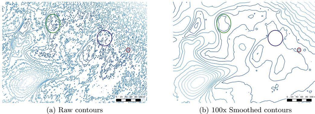
Figure 6: The effect of the smoothing operator on the extracted contours (at every 50cm). The ellipses mark areas where aggregation (green), omission (blue) take place. Note that local maxima as the one indicated by the red ellipse are preserved.
