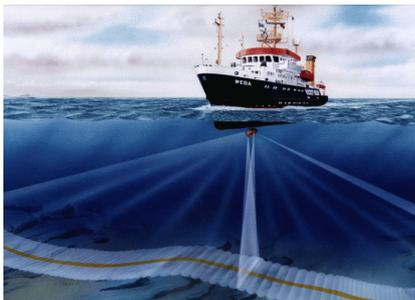
(a) Multi Beam Echo Sounding (MBES) is based on the principle of measuring the time of flight of hundreds of individual signal pulses.
