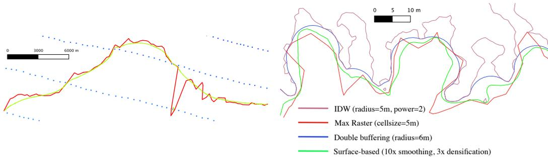
(a) Densification: Comparison of corresponding contour lines. The red line is derived from a surface that was not densified, the green line is derived from a surface that was densified 3 times. Also shown are the sample points in blue.
