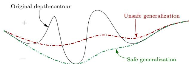
(b) During generalization, contours can only be moved towards greater depth, indicated by a '-', in order to respect the safety constraint.
