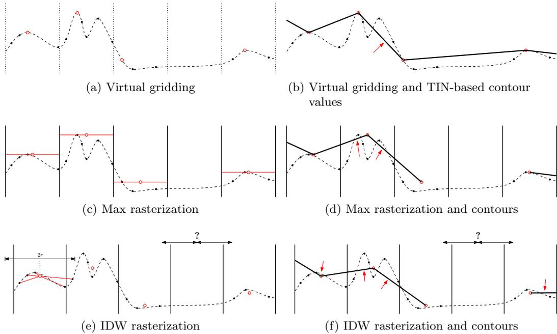
Figure 3: On the left: profile views of different filtering and rasterization methods. On the right: the corresponding contours. Red arrows indicate where the safety constraint is violated with respect to the original points. Also note that in case a grid cell contains no data, no contours can be derived.
