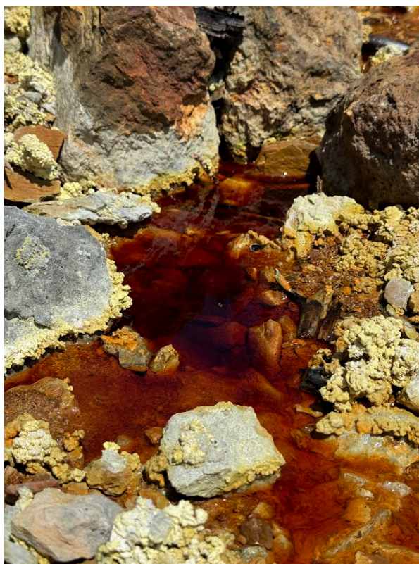
Figure 1.8: Acid Mine Drainage observed in the study area during Q4 2024 fieldwork.
