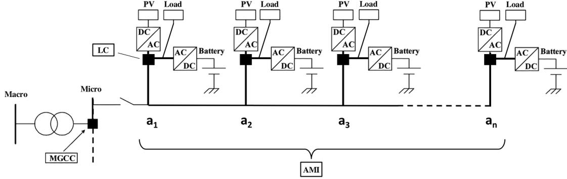
**Figure 2-1:** Simplified lay-out of a micro-grid. LCs are tasked with primary control, where behind the DER reside, linked by bi-directional AC/DC converters.  $E_{\text{consumption}}$  originates from the load,  $E_{\text{production}}$  from its PV panels and  $SOC_{\text{actual}}$  from the battery. All households in the community are communicating with each other using an AMI network.
