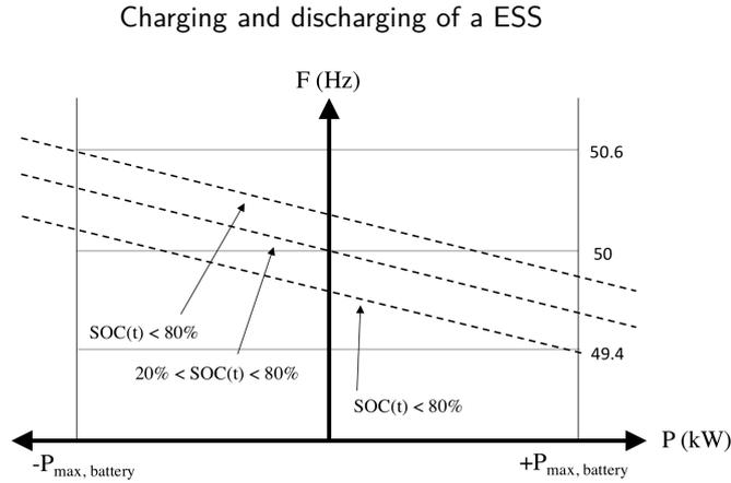
**Figure 2-5:** ESS units manage their charging and discharging behaviour by shifting their droop-parameter upwards or downwards with respect to the prime-mover  $\omega_n$ .  $\omega_{\text{ESS}}$  has to stay within bounds of European standards [49.9, 50.1] in Hertz and cannot exceed its power limits [ $P_{\min}$ ,  $P_{\max}$ ]
