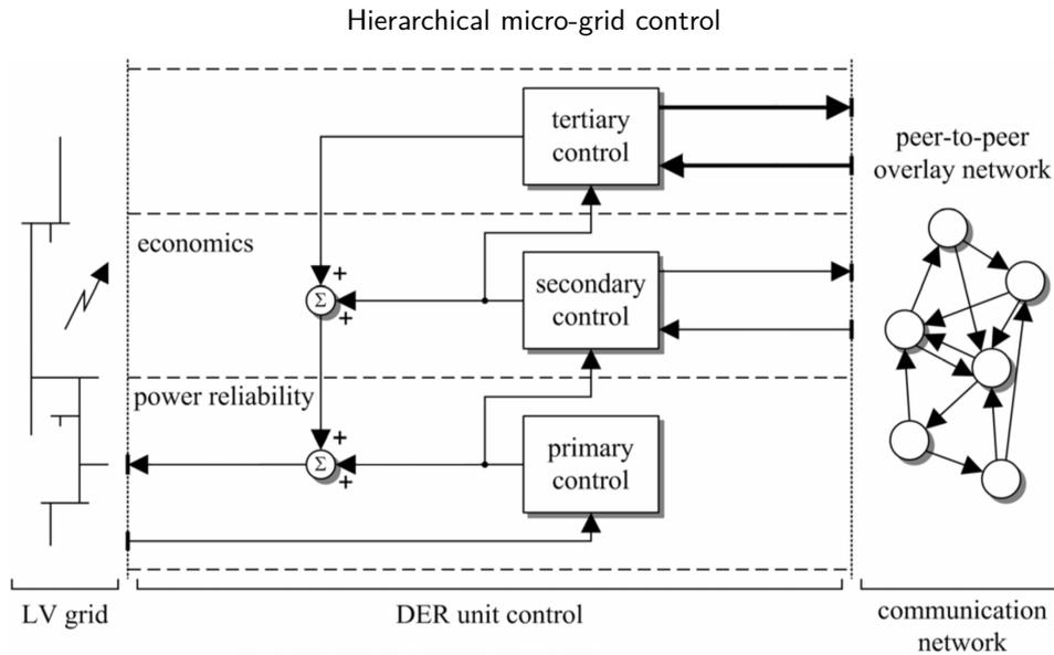
**Figure 2-2:** A DG unit utilizes a three-folded control decoupled structure. Standalone primary control has fast sample time/dynamics and does not communicate with neighbors. Secondary control governs energy dispatch at a larger timescale, with higher sampling time and slower dynamics. Tertiary control is involved in the day-to-day markets. From a micro grid perspective, tertiary control governs connection to the macro-grid.
