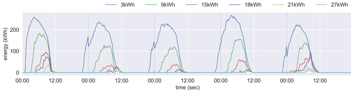
**Figure 4-3:** Influence of battery sizes on total deficit: by increasing the maximum battery capacity, deficits in the micro-grid decrease. The rate of deficit reductions slows down with higher battery sizes. On default, we chose a battery size of 19 kWh.
