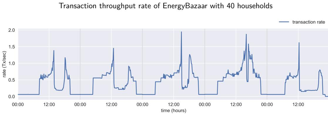
Figure 4-13: Transaction rate of agent communication to the Blockchain. Maximum transaction rate is  $\approx 2$  Tx/sec for a micro-grid of 40 households.
