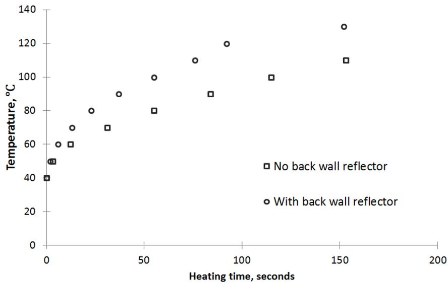
Figure 5. Experimental dependencies of glucose syrup temperature from time of laser heating (with and without reflection from back wall).
