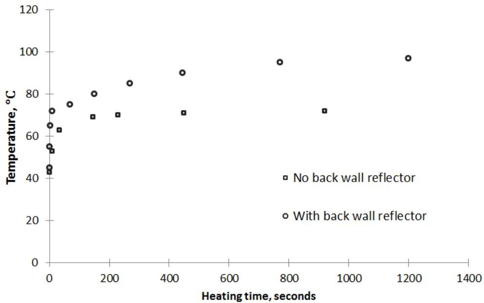
Figure 4. Results of experiments with laser heating of vegetable fat with and without reflection from back wall.
