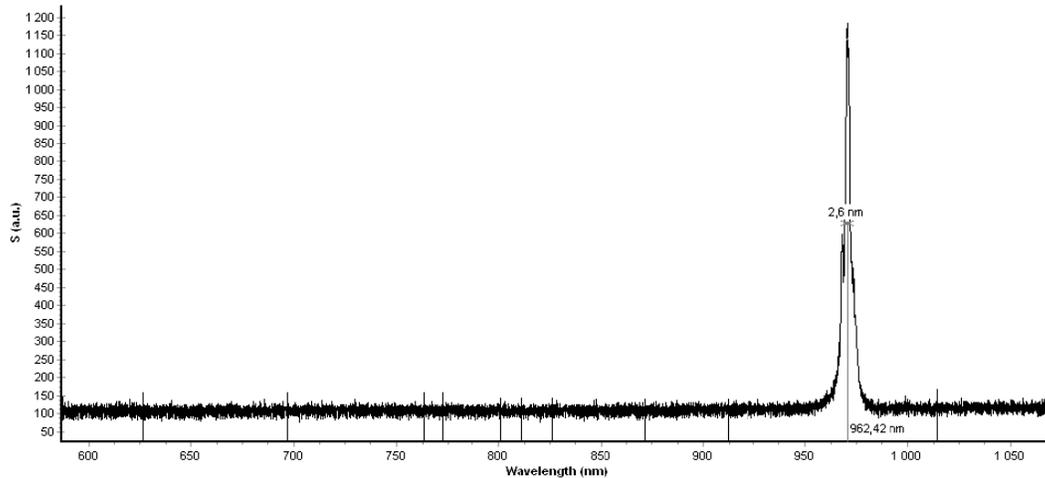
Figure 2. Radiation spectrum of laser diode used in experiments.
