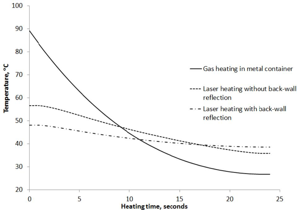
Figure 3. Simulated temperature distribution with average temperature of 45°C for heating in metal container with gas heater, laser heating with and without back-wall reflector.
