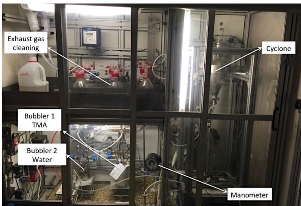
**Figure 2-3:** ALD setup used in the experiment.
