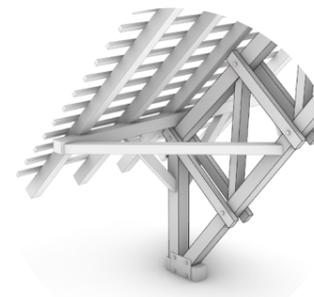
Zoomed in detail of the bottom of the timber truss transferring load to masonry walls below (modelled by author)
