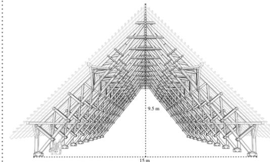
Above: an axonometric view of a single Truss member with the supported roof plane - an assembly of standardized dimensioned timbers.
