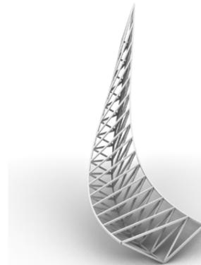
An isolated single piece of spiral timber spaceframe - the entire structure consists of 20 of such assemblies.
