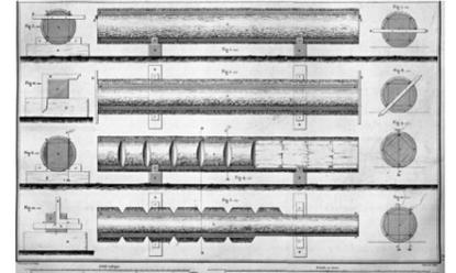
Diagram showcasing how trunk is turned into a beam (source: Emy 1841)
