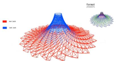
Parametric model adapted by engineers specifying distribution of 4x4's and 2x4's to optimise the structure (formatengineers.com, access: 05.01.2022)
