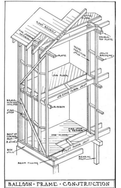
An infographic presenting standardised Balloon Frame construction system (source: Holman 1929)
