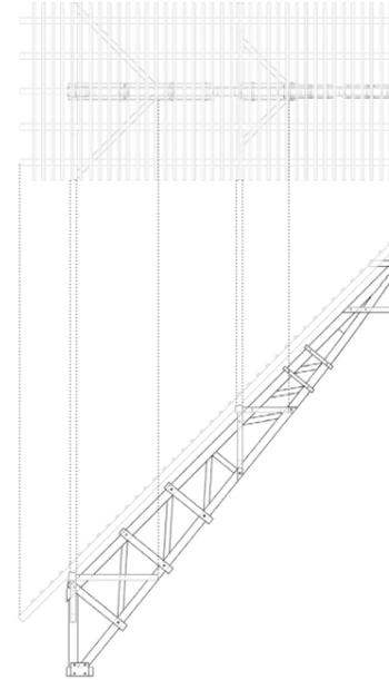
Single truss - a key standardised and repetitive structural element in plan and elevation (drawn by an author)
