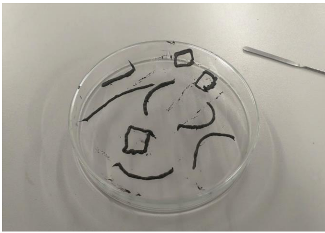
Figure 4.34: Shapes created with the use of the electromagnet curled up upon themselves immediately after taking off the cured silicone from the glass (build) plate.
