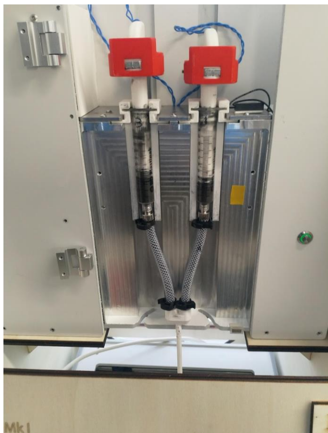
Figure 4.57: 10 cm long tubes were used to test a new static mixing nozzle design, which ended up proving magnetic material could be extruded when making use of very short transport tubes.
