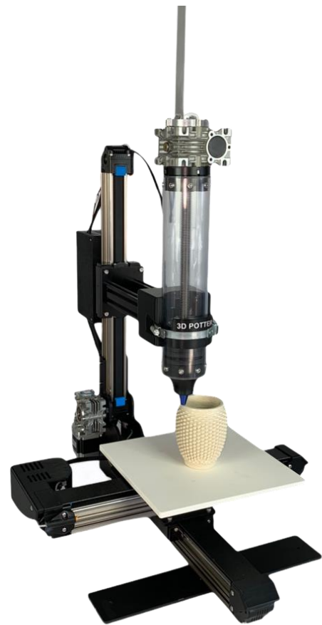
Figure 4.63: Another paste printing solution by +Lab, which uses a large gear ratio to generate enough pressure to extrude thick paste materials. The 3D printer used here has a stationary head (Milkert, 2014).
