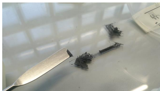
Figure 4.53: At every attempt, the printed samples did not cure because of a wrong A/B ratio.
