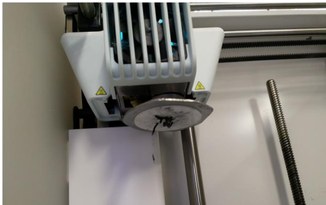
Figure 4.44: When too large, the magnetic shield would jam into the motor shrouds in the corners of the 3D printer, potentially breaking the static mixing nozzle to which it is attached.
