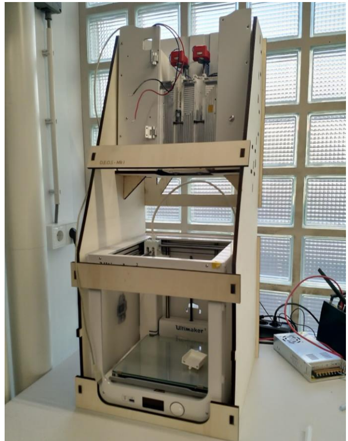
Figure 4.41: The designed overhead support structure allowed the extrusion system to be placed 20 cm above the printhead.
