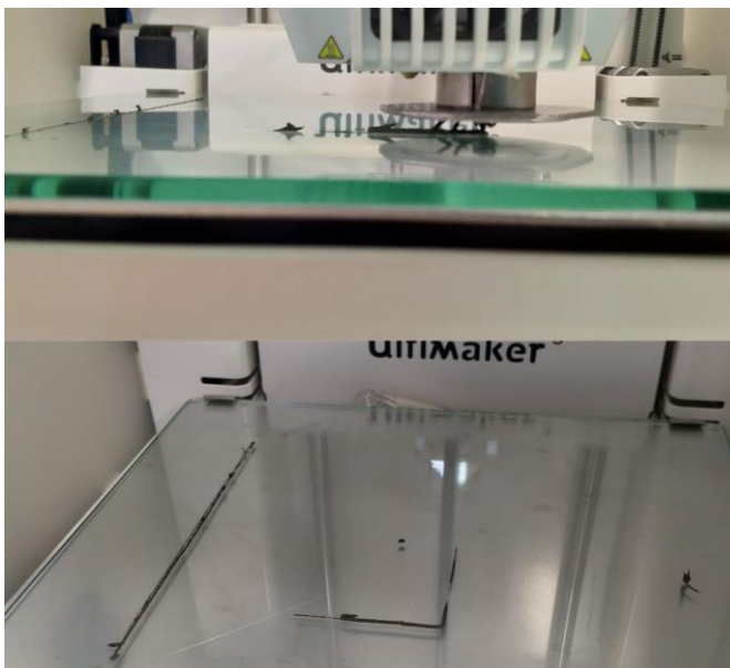
Figure 4.50: With all implemented modifications, magnetic ink was able to be extruded. However, this was no smooth experience, of which the attraction of ink by the magnet despite the shielding is just one example.
