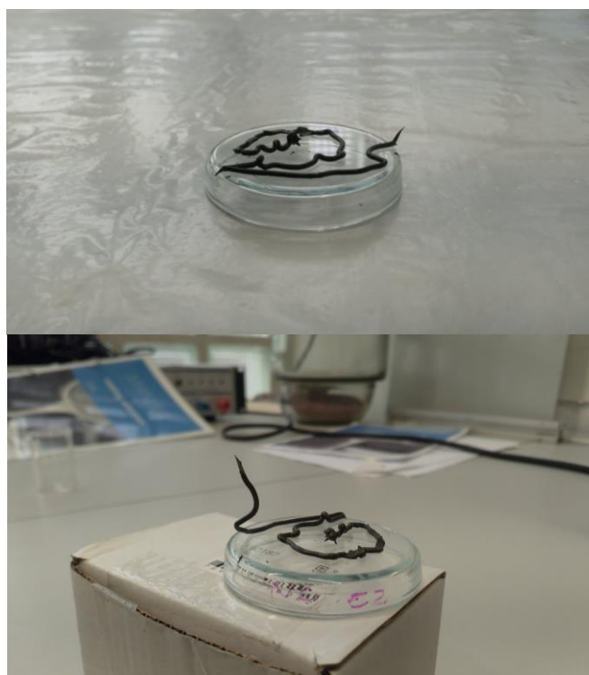
Figure 4.58: A scribble could be 4D printed when using 10 cm tubes and showed good magnetic response.
