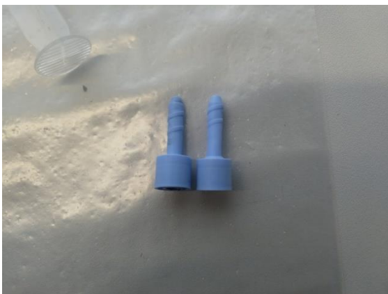
Left: new nozzle, right: used nozzle deformed by heat of electromagnet.
