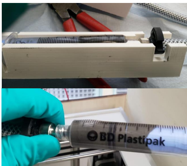
Figure 4.51: Because of the high pressure, syringes started swelling, leading to under extrusion of ink.
