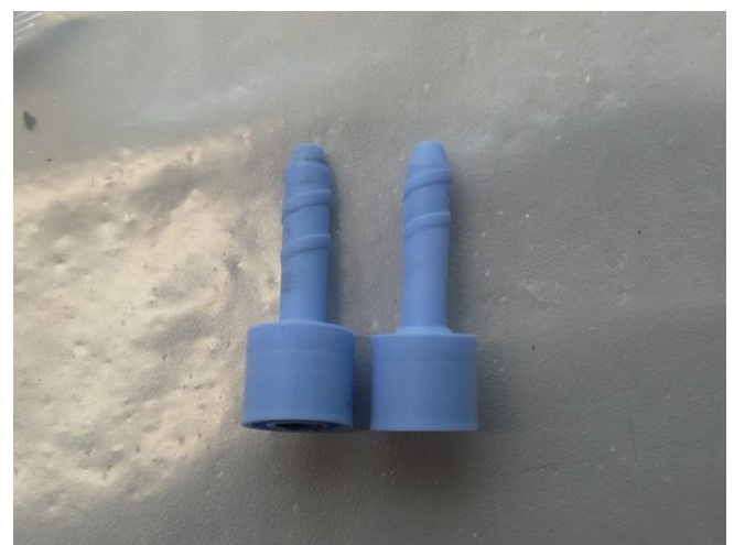
Figure 4.33: The heat generated by the electromagnet was enough to make the PLA nozzle piece soft, which caused it to elongate, get thinner and crooked (right). Left, an unused piece can be seen.
