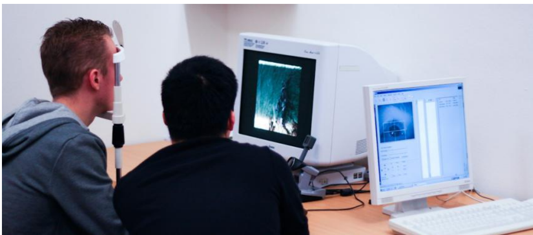
Figure 3.1: Experimental setup showing the participant (left) with his head on the chinrest. The experimenter (middle) can follow the experiment and control the eye tracker from the screen on the right. The eye tracker itself can be seen at the bottom-right of the participant's screen [59].
