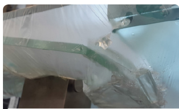
Image 3: panel penetrated by the support
