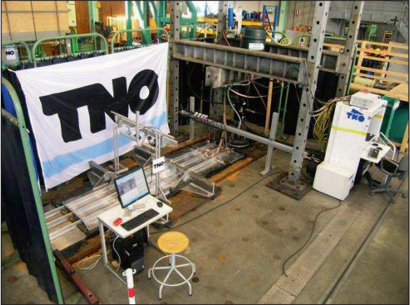
Figure 5.56: LSS layout and fatigue test setup
