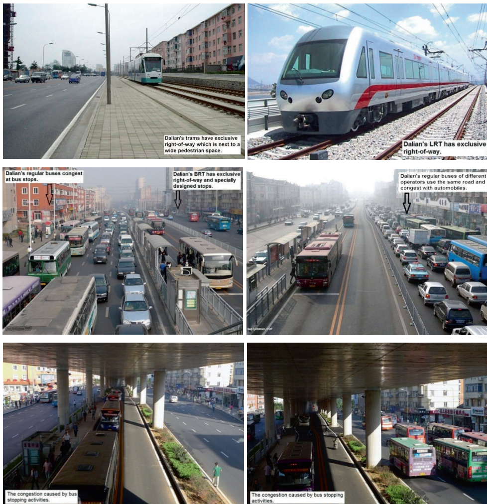
Figure 6.13 Exclusive right-of-way versus mixed right-of-way
