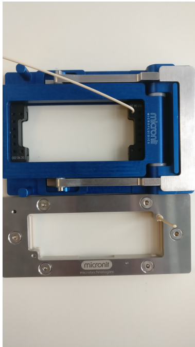
Fig. 33. The original Micromodel Holder and the newly designed micromodel holder with top view. Where the new holder has screw to clam the Peek tubing
