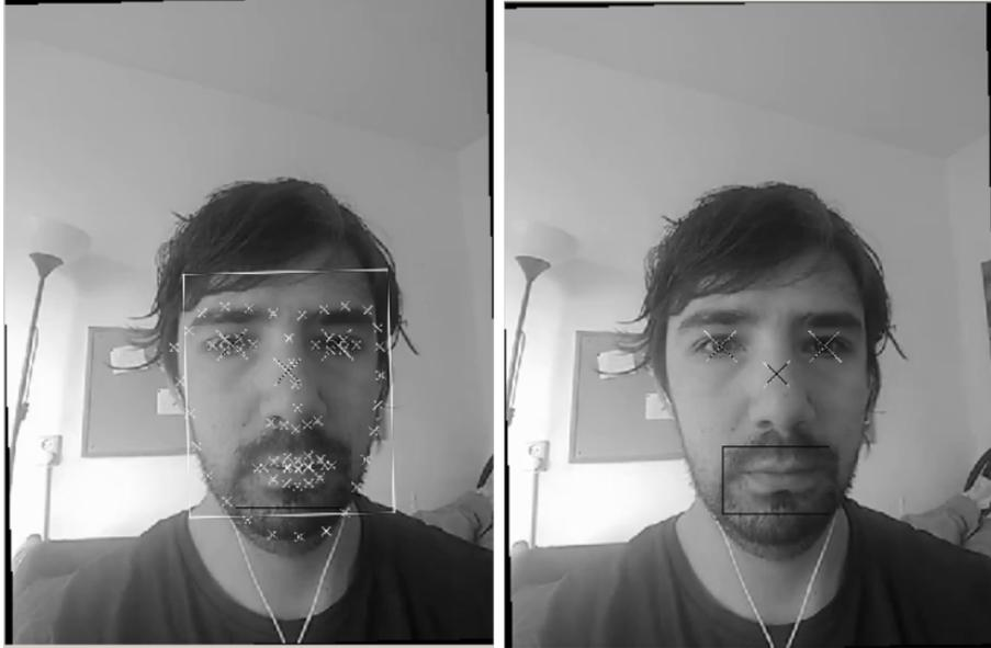
Figure 4.1: Landmark position and face correction for mouth tracking. (left) Bounding box face and landmark position. (right) Eyes and nose points used for mouth bounding box.
