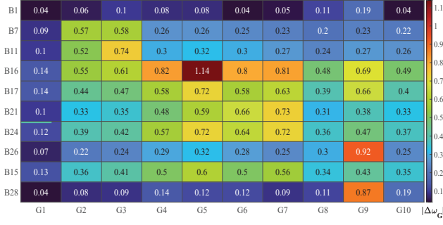
Figure 1. Case study shows the variation in rotor angle ( \Delta\omega_G ) of Generators numbered G1 to G10 when subjected to Fault at different buses (B#).
