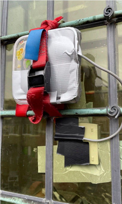
PLACEMENT LOGGERS CLOSED CAVITY WINDOW TEMPERATURE GLASS OUTSIDE & INSIDE & CAVITY
