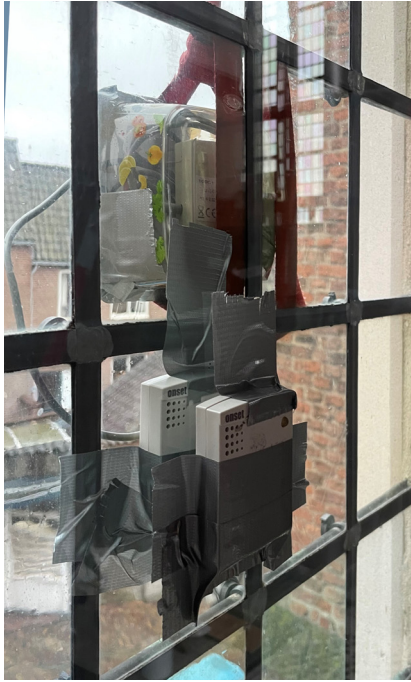
PLACEMENT LOGGERS CLOSED CAVITY WINDOW TEMPERATURE GLASS OUTSIDE & INSIDE & CAVITY
