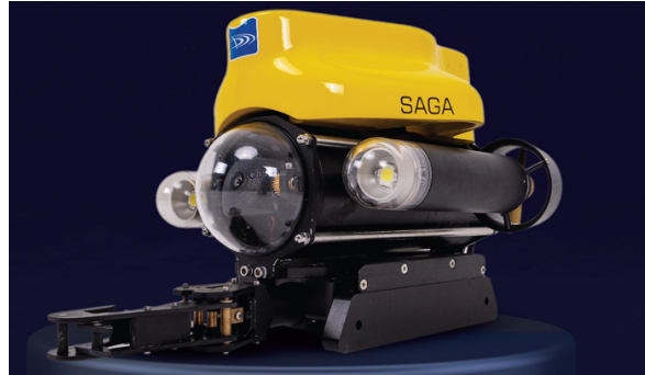
Figure 3-10: Image of the real Desistek SAGA ROV used in simulation. The model is sourced from [21].
