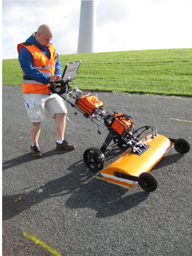
Figure 6. IDS 8-channel GPR survey equipment.
