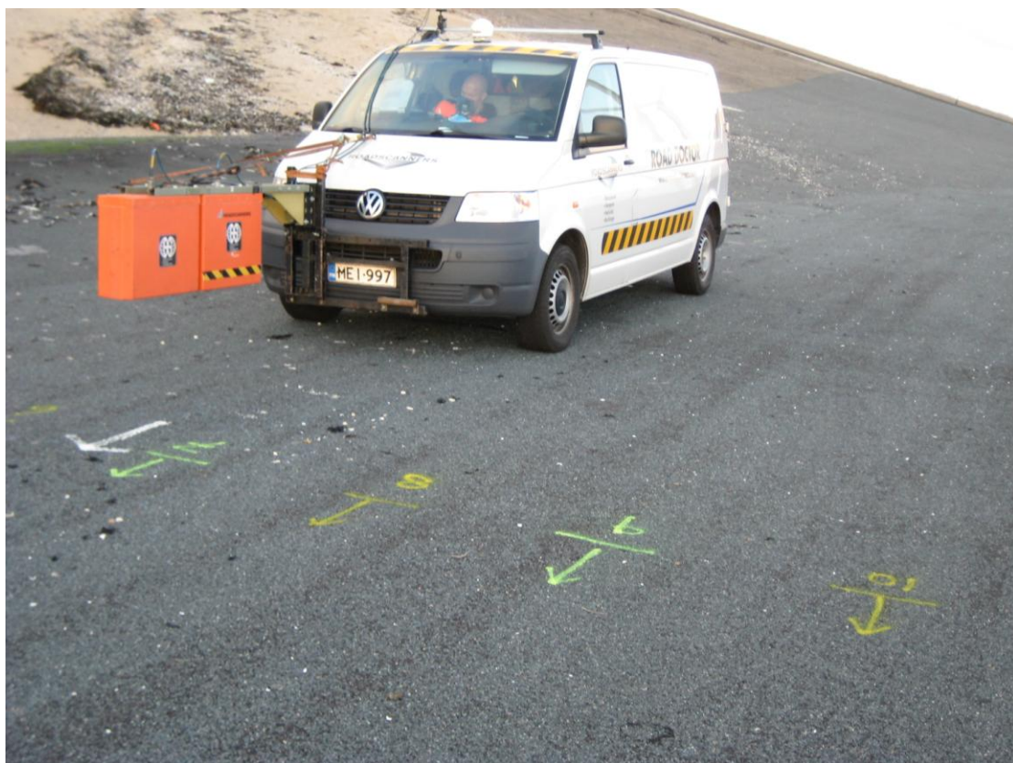
Figure 5. Survey van equipped with GSSI 1.0 GHz and 2.2 GHz horn antennas mounted on the same frame.
