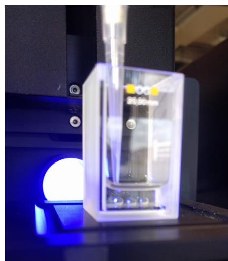
Figure 4-11. Immersed contact angle measurement in the macro-cuvette.
