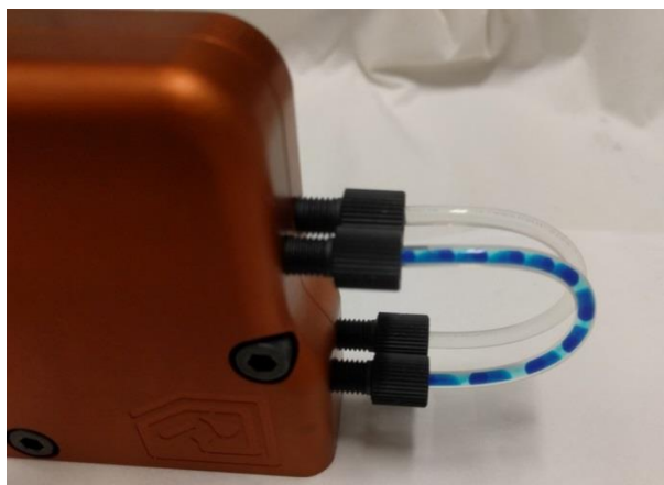
Figure 4-20. Breakthrough of aqueous phase. Light blue is the organic phase, dark blue is the aqueous phase coloured with methylene blue dye. Front tubing is the organic side of the separator, back tubing is the aqueous side of the separator.
