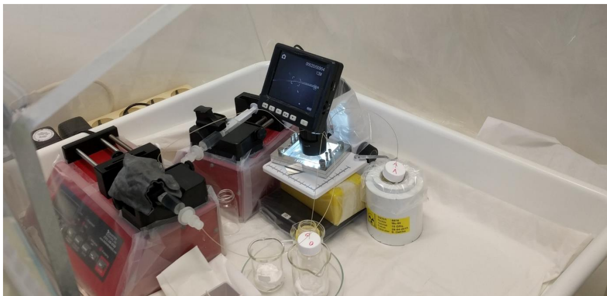
Figure 3-3. Setup for the radioactive extraction on the microchip.
