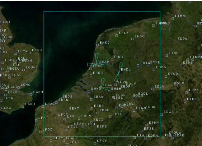
Fig. 1. An overview of the simulated BlueSky environment, showing the blue triangle goal states. The blue rectangle describes the area in which aircraft are generated.
