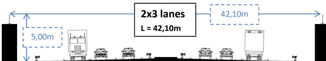
Fig. 37: Profile of the 2x3 lane highway that the bridge could span. The single span would be 42,10 m, if an intermediate support is used, the span would be 2x21,05 m.
