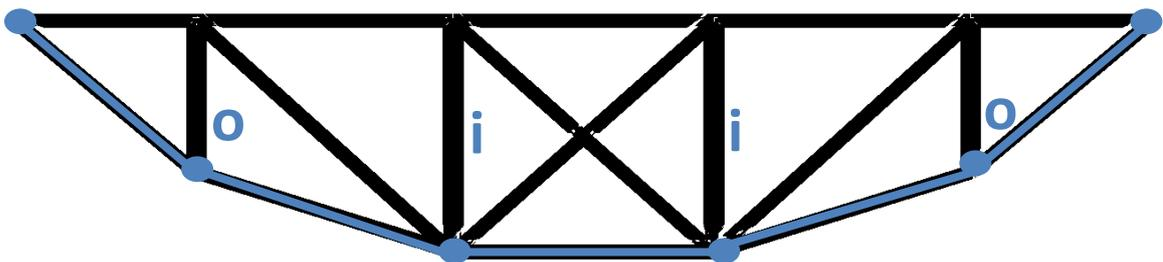
Fig. 108: Topology of the lateral trusses that act as substructure for the inner bridge deck.
