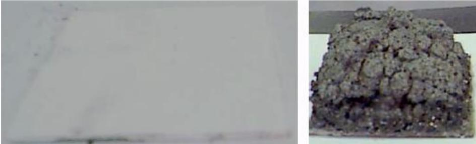
**Fig. 12: Intumescent coating before (left, thickness = 0,8 mm) and after (right, thickness = 52 mm) fire loading [B07, p282]**
