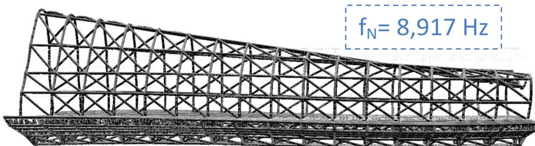
Fig. 149: Mode 4: The second vertical mode. Only the elliptical truss deforms in z-direction at a natural frequency of  $f_N=8,917$  Hz.
