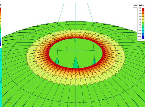
Figure 173: Stresses around edge after improvements and raising thickness
