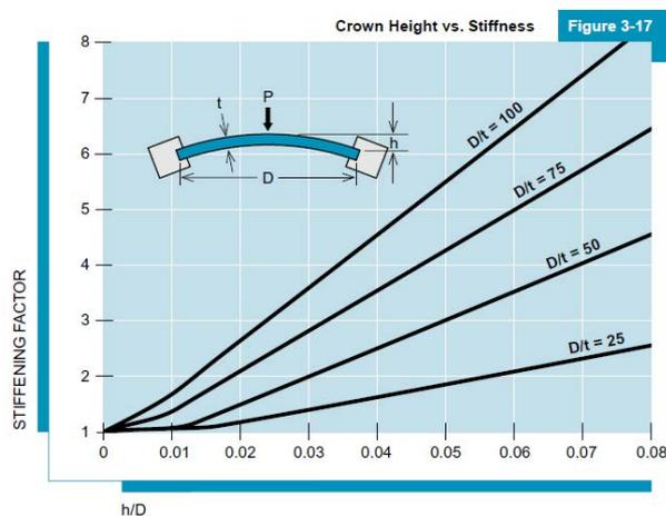
Figure 71: Increase of stiffness for curved plates (Bayer 2001)
