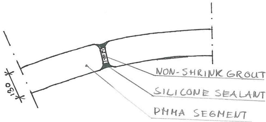
Figure 204: Subsurface room wall segments
