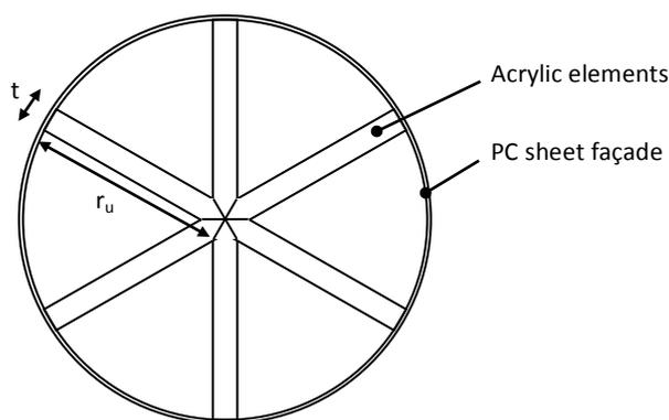
Figure 126: Star shaped bearing structure (cross-section).
