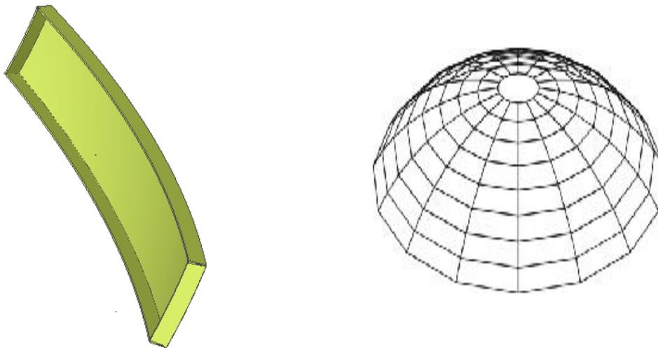
Figure 163: Possible segment (left) and deviation of the sphere (right) for a ribbed dome
