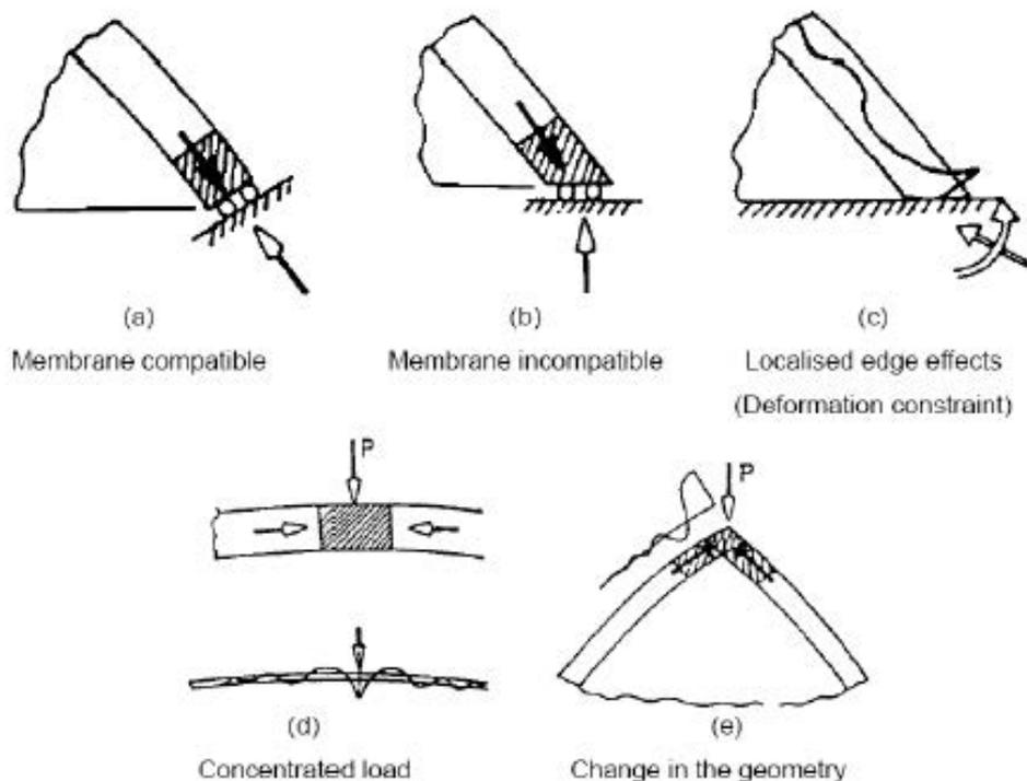
Figure 146: Membrane theory compatibility conditions in a shell. (Maten 2011)
