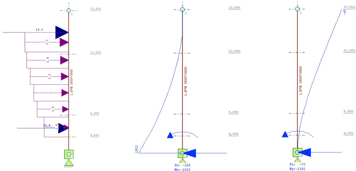
Figure 134: Deformation caused by wind forces as calculated by Technosoft<sup>1</sup>.
