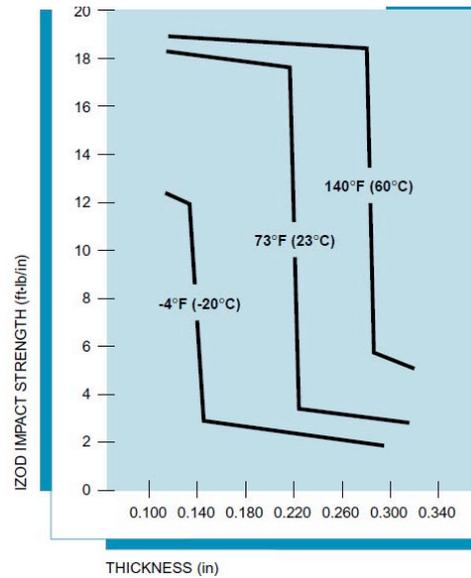
Figure 65: Critical Thickness for polycarbonate walls. (Bayer 2001)
