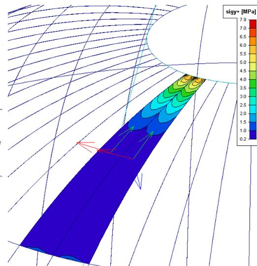
Figure 210: Meridional stress in top segment for load case ULS 2
