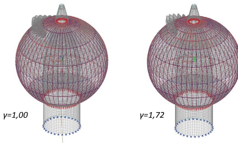
Figure 181: Safety factor and buckling before (left) and after (right) optimization
