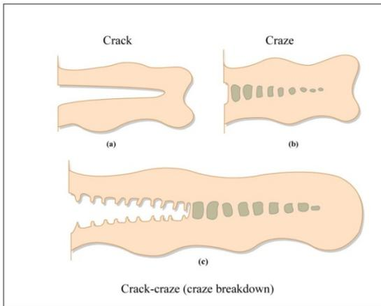
Figure 66: Principles crack and craze (MIT 2012)
