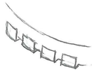
Figure 207: 3D view part of the steel ring with support-hands
