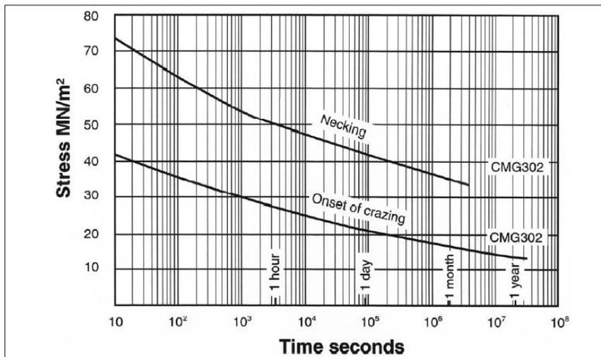
Figure 5 Static fatigue characteristics at 23°C, 65% rh
