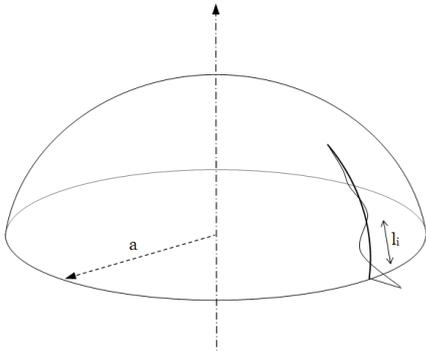
Figure 147: Edge disturbance and influence length for a dome structure
