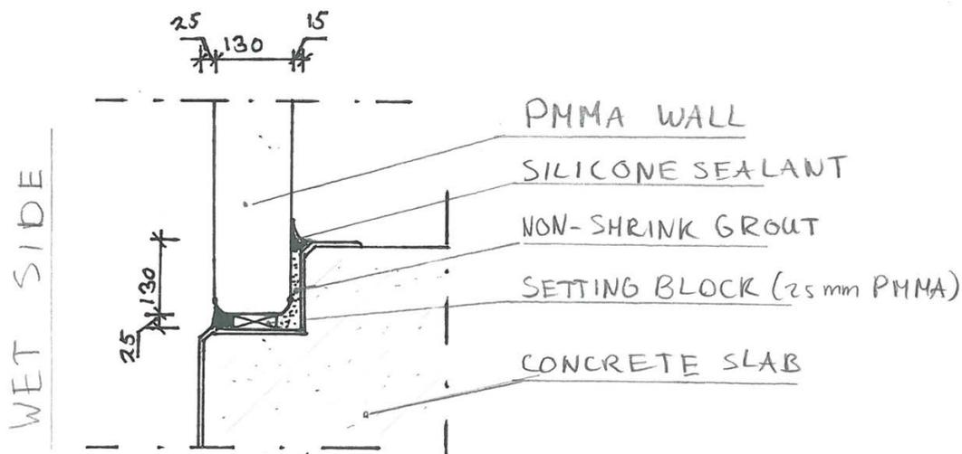
Figure 216: Joint subsurface PMMA wall and concrete foundation
