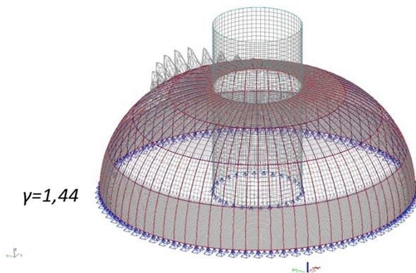
Figure 184: Buckling behaviour of the dome structure for UGT4b
