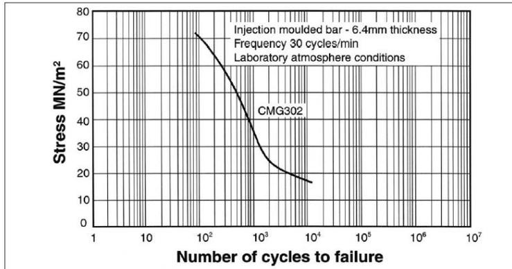
Figure 6 Dynamic fatigue characteristic in flexure at 23°C, 65% rh
