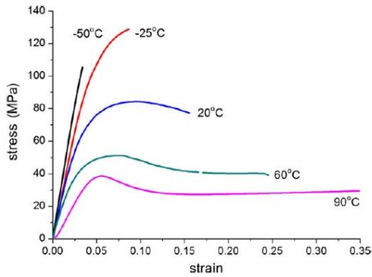
Figure 46: Stress-strain graphs for PMMA (Liu 2008)
