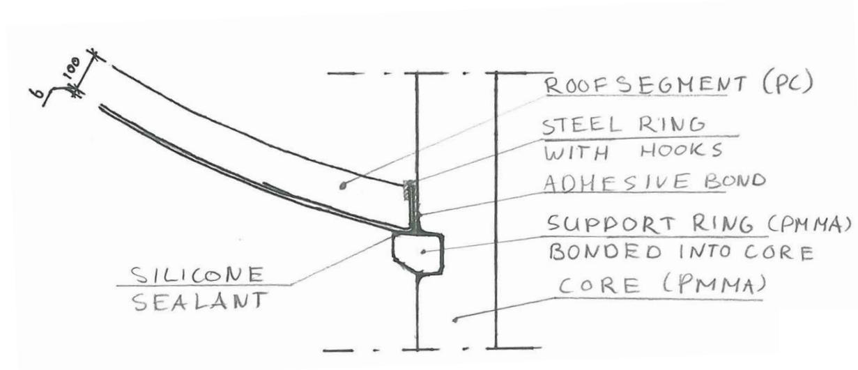
Figure 211: Section of joint Polycarbonate segment to the core, bottom of the sphere
