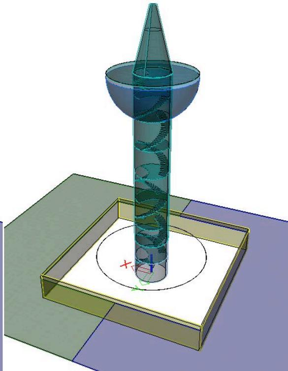
Figure 225: Step 8: The conical core element.
