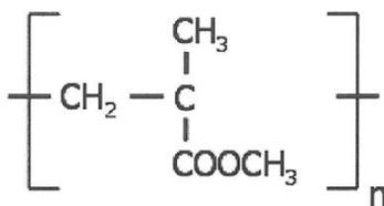
Figure 10: Structure PMMA
