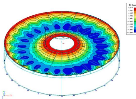
Figure 191: Maximal vertical deflection of the floor
