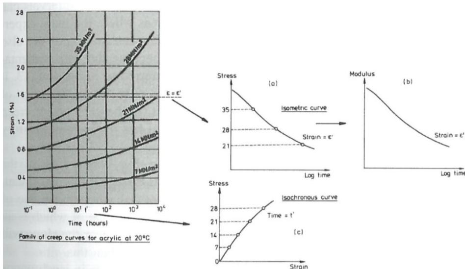
Figure 42: Creep behaviour of PMMA (Crawford 1998)
