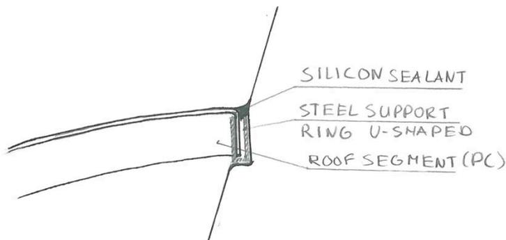
Figure 208: Section PC roof segment to core joint, top of the sphere
