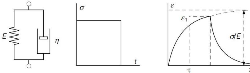
Figure 35: Creep behaviour of the Kelvin-Voigt element (Vegt 1991)
