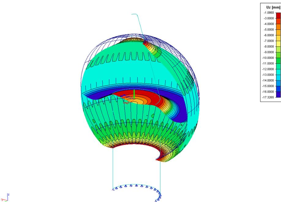
Figure 176: Vertical deformations, BGT2
