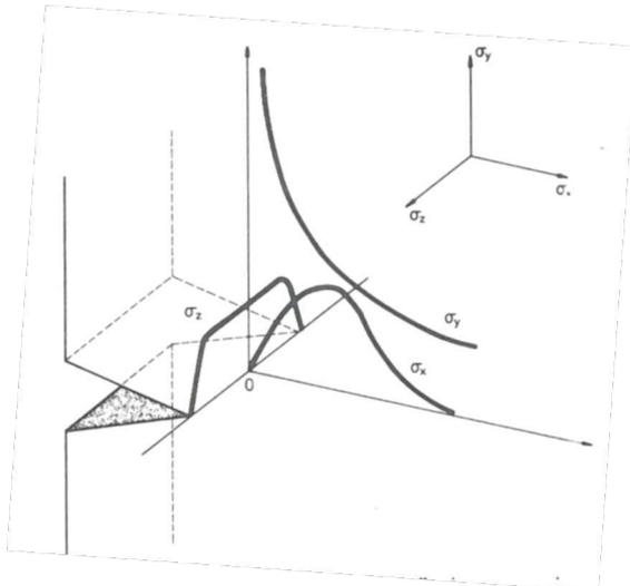
Figure 68: Tri-axial stress developing around crack (Crawford 1998)
