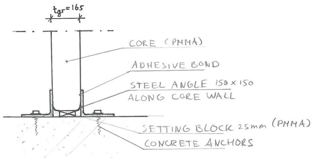
Figure 215: Connection of core parts to the concrete foundation
