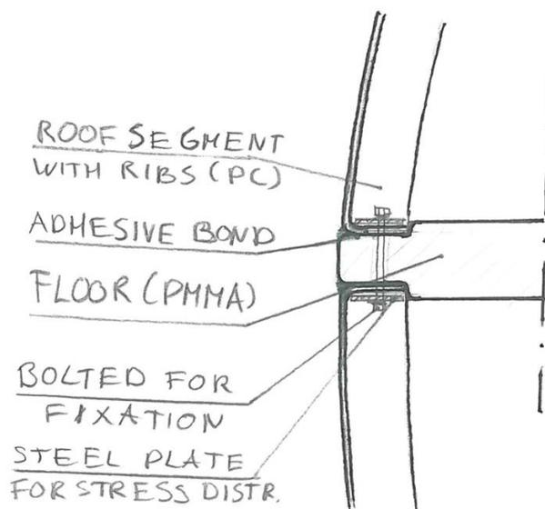
Figure 214: Joint between sphere and observatory floor
