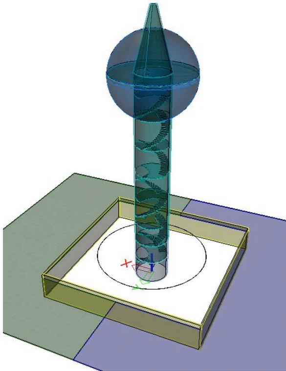
Figure 226: Step 9: Upper half of the sphere
