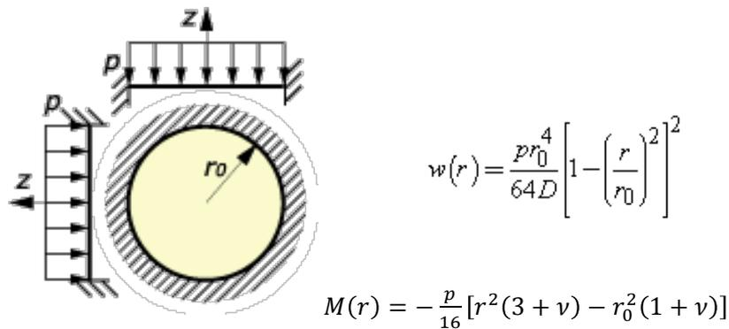
Figure 193: Moments and deformations for clamped circular floors (efunda.com)
