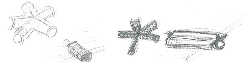
Figure 157: Nodes for connecting struts.
