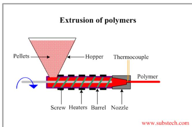
Figure 16: Extrusion process
