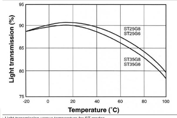
Figure 55: Transparency versus temperature (Lucite 2001)
