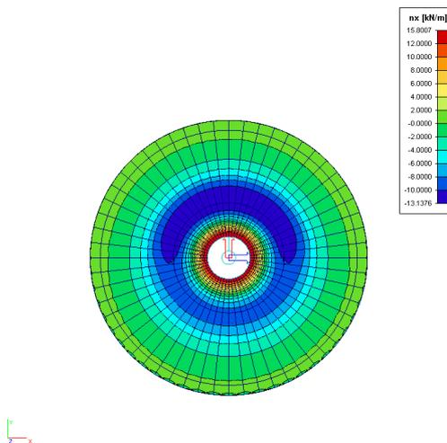
Figure 179: Membrane force nx sphere structure for UGT4b
