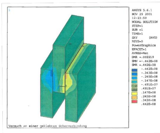
Figure 81: Stress distribution in a glued PMMA samples (Gleiter 2002)
