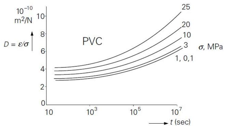
Figure 30: Non-linear behaviour of plastics; change of modulus in time for several stress levels of PVC (Vegt 1991)
