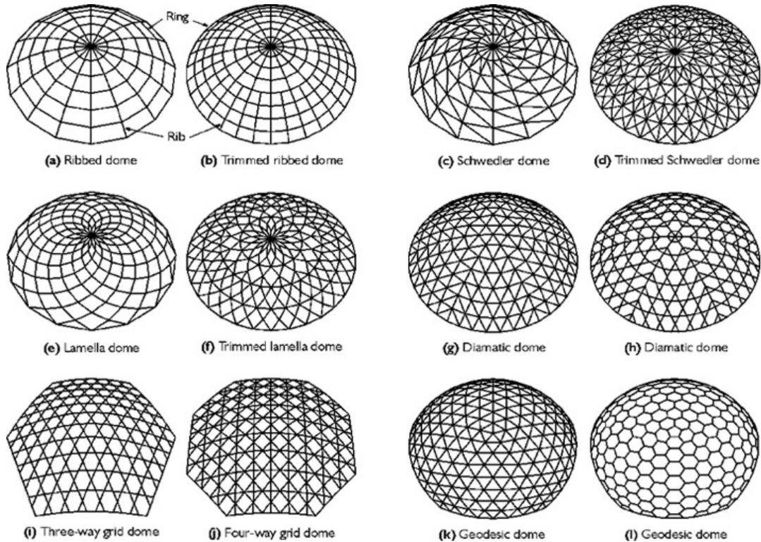
Figure 153: All kinds of possibilities to create a dome structure
