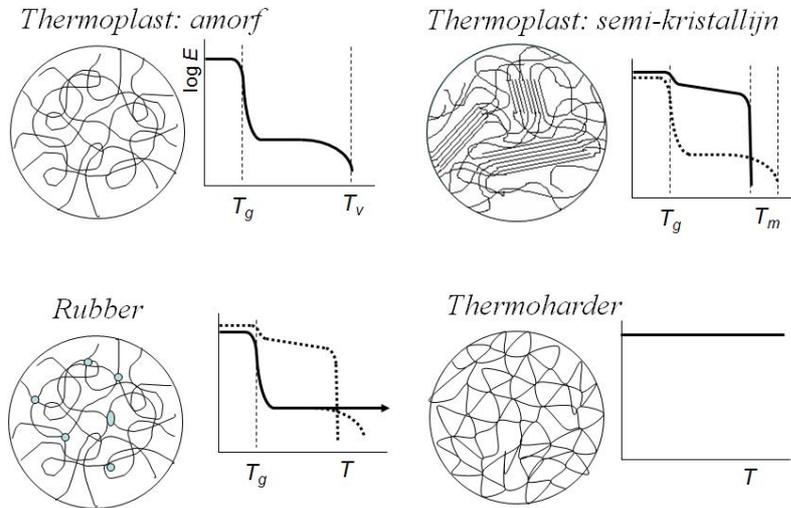
Figure 7: Difference between polymer subtypes
