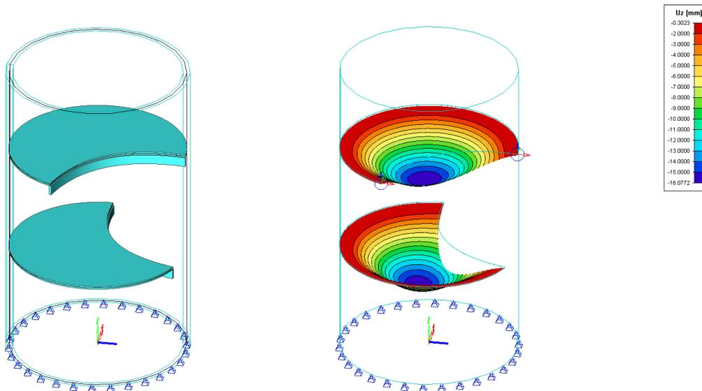
Figure 196: Final design landing lay-out and resulting deformations
