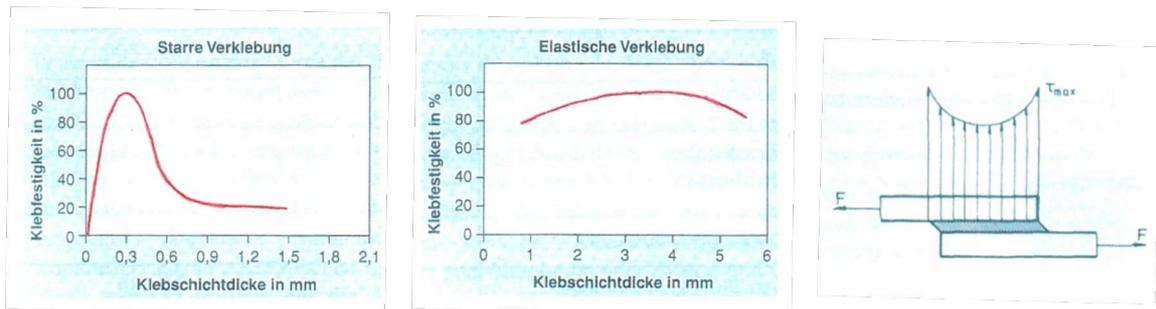
Figure 79: Relation between relative adhesive strength and adhesive thickness for a stiff and a flexible joint (Gleiter 2002)
