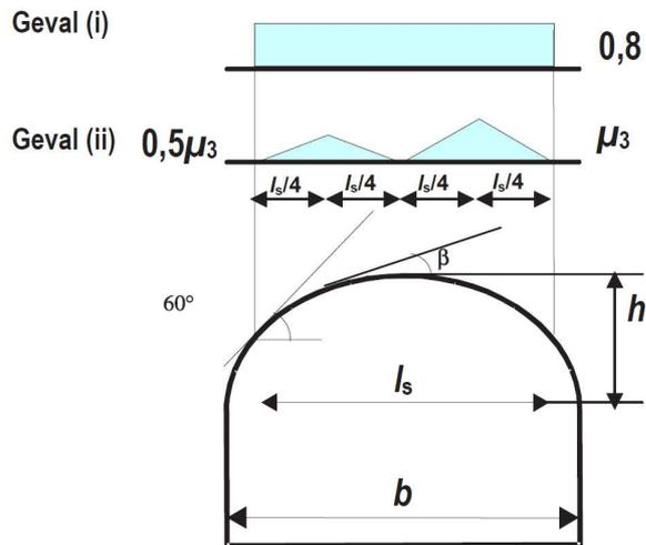
Figure 105: Snow load coefficients for cylindrical roofs. (NEN-EN1991-1-3 2003)
