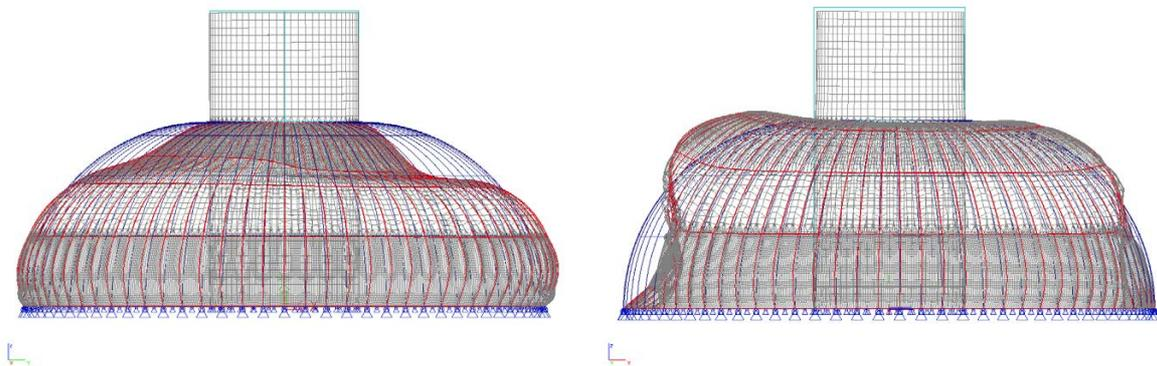
Figure 178: Deformation behaviour of the dome for BGT4b (left) and BGT3 (right)
