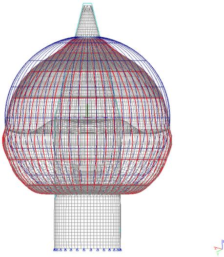
Figure 174: Deformed structure, loadcase UGT2
