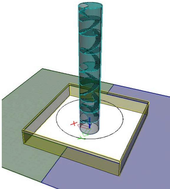
Figure 222: Step 5: Rest of the core is installed likewise
