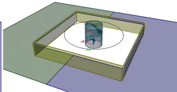
Figure 221: Step 4: Stacking the next core section, stairs and landing
