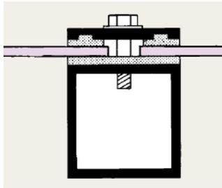
Figure 89: Example of a clamped connection, window frame. (Röhm 2002)
