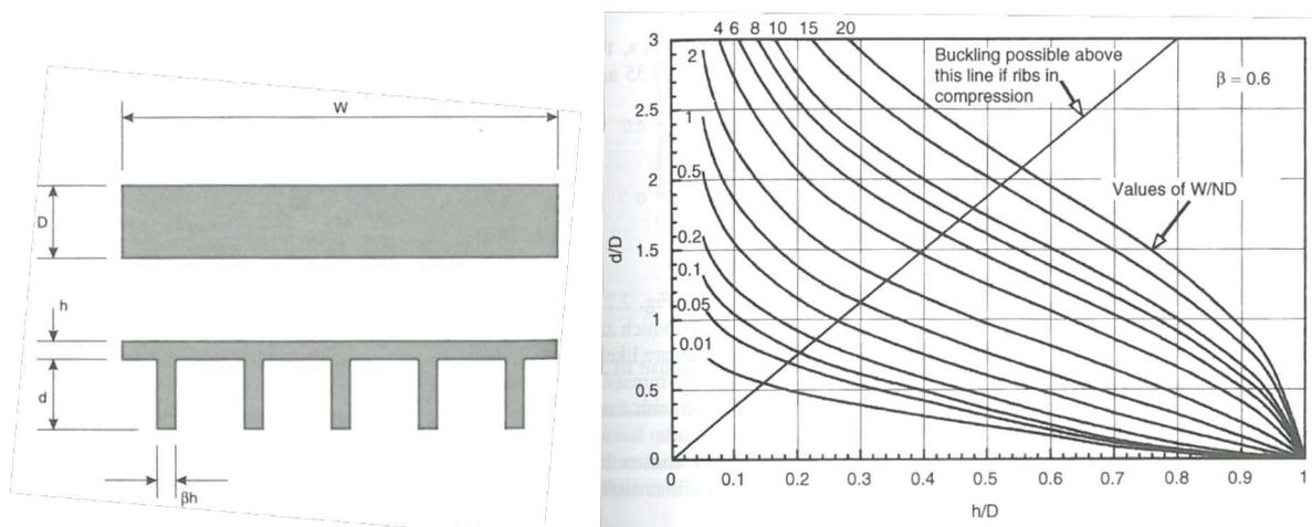
Figure 72: Design of ribbed plates (Crawford 1998)
