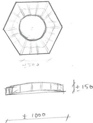
Figure 158: Injection moulded element with ribs and a circular rib-free 'window'
