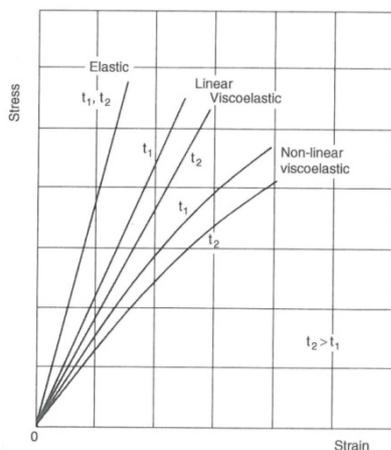
Figure 29: Stress-strain graphs for elastic and (linear and non-linear) viscoelastic behaviour at two points in time (Crawford 1998)
