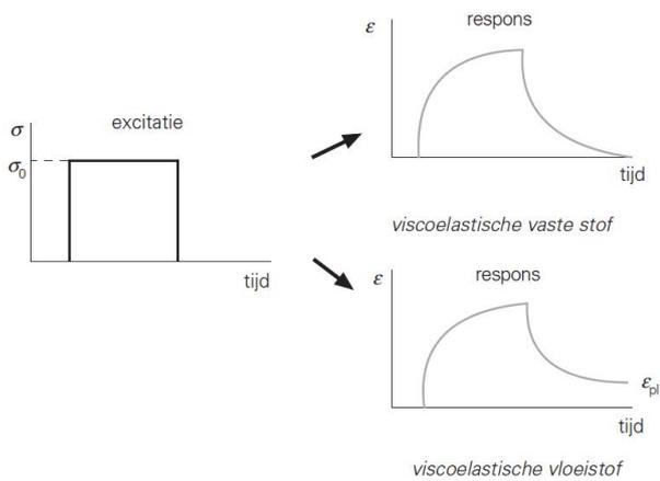
Figure 31: Response of a viscoelastic solid and fluid to a constant stress (Vegt 1991)
