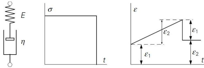
Figure 33: Response of Maxwell model to constant stress – creep (Vegt 1991)
