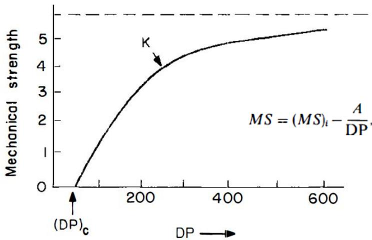
Figure 5: Tensile properties as a function of molecular weight of DP (Atlas 1976)
