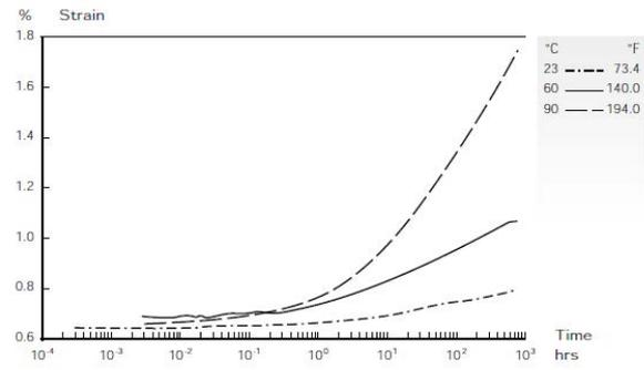
Figure 41: Strain in time for different temperatures PC (at 15 MPa) (GE Plastics 2004)
