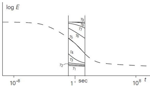
Figure 91: Mastercurve (Vegt 1991)
