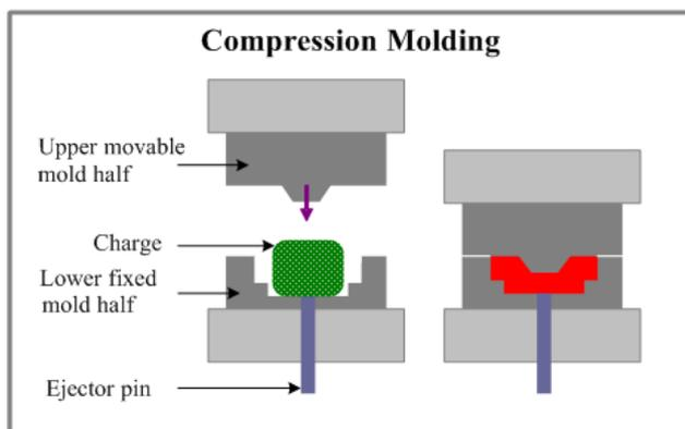
Figure 18: Compression moulding
