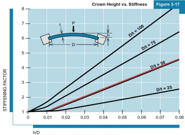
Figure 160: Crown height vs. Stiffness
