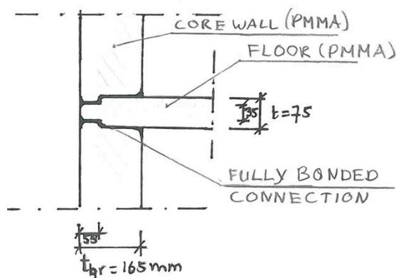
Figure 200: Floor integrated in the core wall
