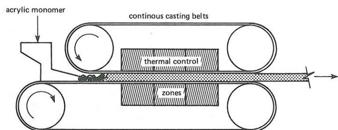
Figure 15: Continuous casting
