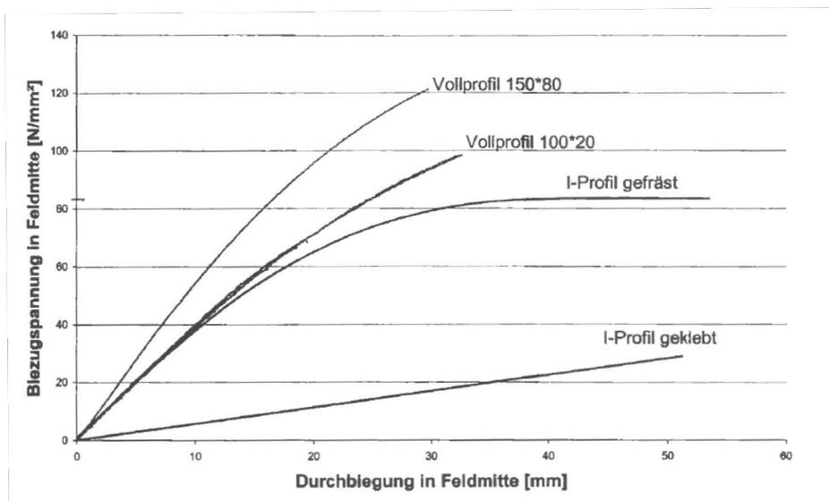
Figure 76: Results of the 4 points bending test for various shaped PMMA profiles (Gleiter 2002)
