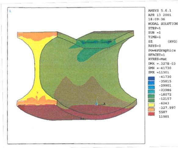
Figure 74: Improved I profile, milled (Gleiter 2002)
