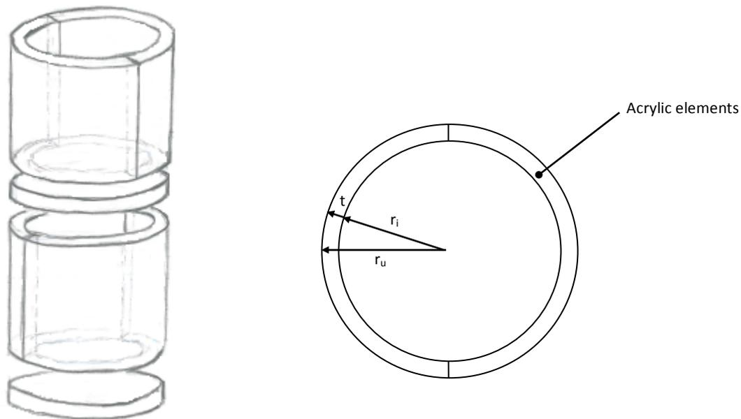
Figure 128: left: Side view of stacked tube structure; right: cross section of the bearing structure (core).
