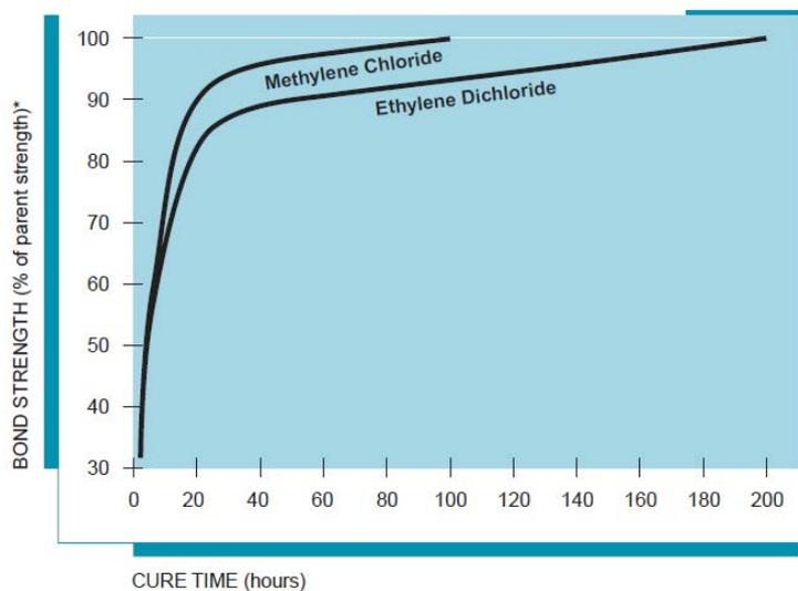
Figure 83: Influence of post curing on bond strength for polycarbonate (Bayer 2001)
