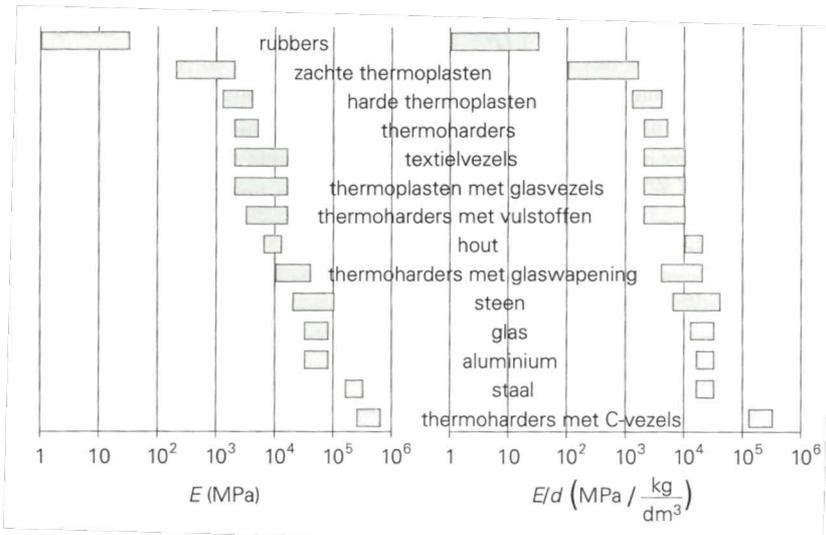
Figure 99: Absolute and weighted modulus of various (building) materials (Vegt 1991)
