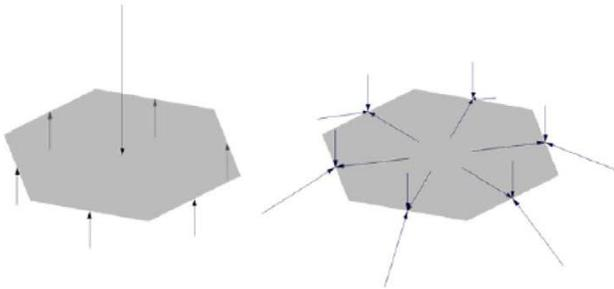
Figure 155: Mechanism of local bending of facets in a shell.
