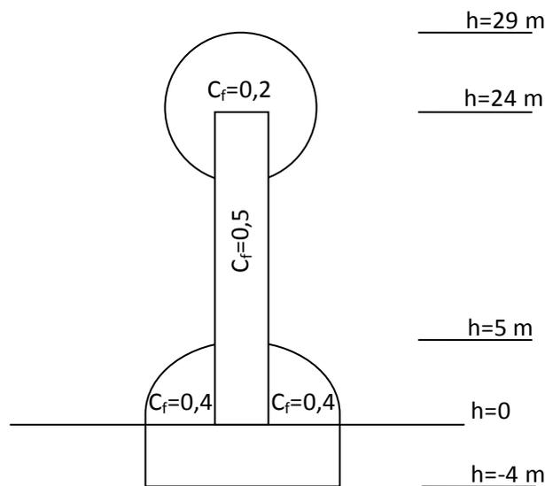
Figure 129: side profile with according wind load factors
