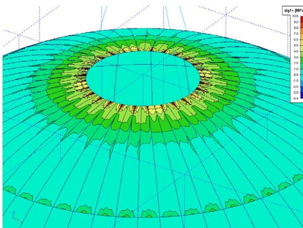
Figure 172: Stresses around edge before mesh refinement and raising thickness
