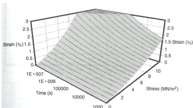
Figure 39: Example stress-strain-time curves (Crawford 1998)
