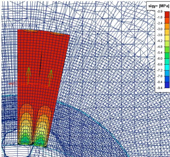
Figure 212: Meridional stresses in lowest sphere segment for load case ULS 2
