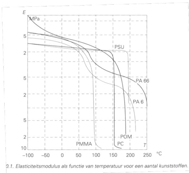
Figure 44: Modulus as function of temperature for several polymers (Vegt 1991)
