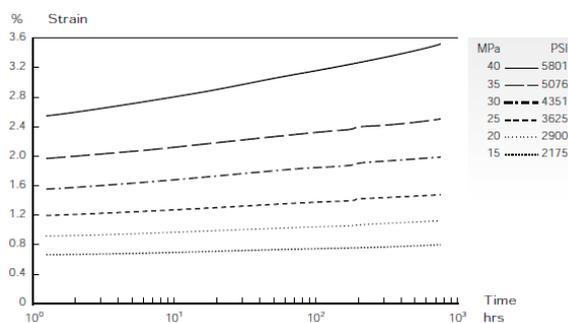
Figure 1: Strain in time for different stresses PC (at 23 °C) (GE Plastics 2004)
