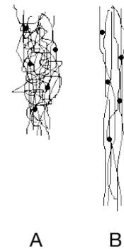
Figure 9: Stretching of elastomers
