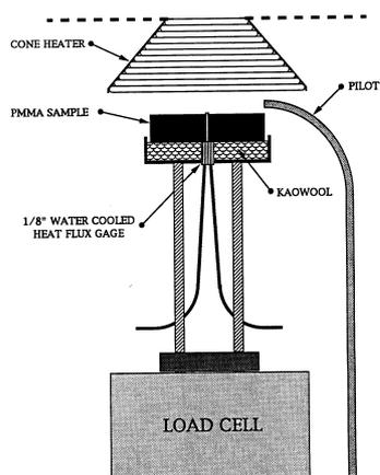
Figure 3.1. Schematic layout of burning rate apparatus
