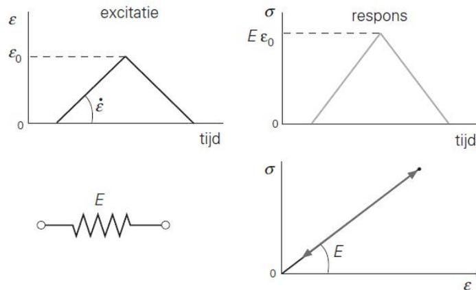
Figure 26: response of elastic material on a constant strain rate (Vegt 1991)
