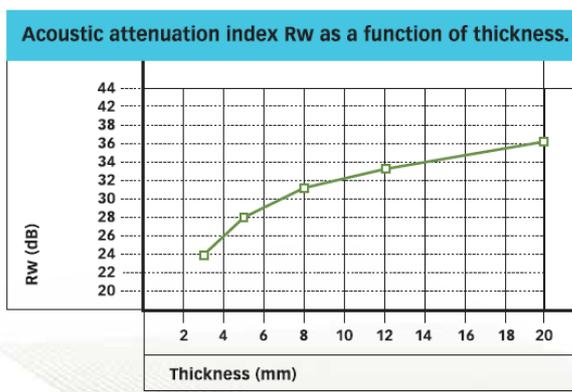
Figure 56: Sound Reduction as function of thickness (Altuglas 2005)
