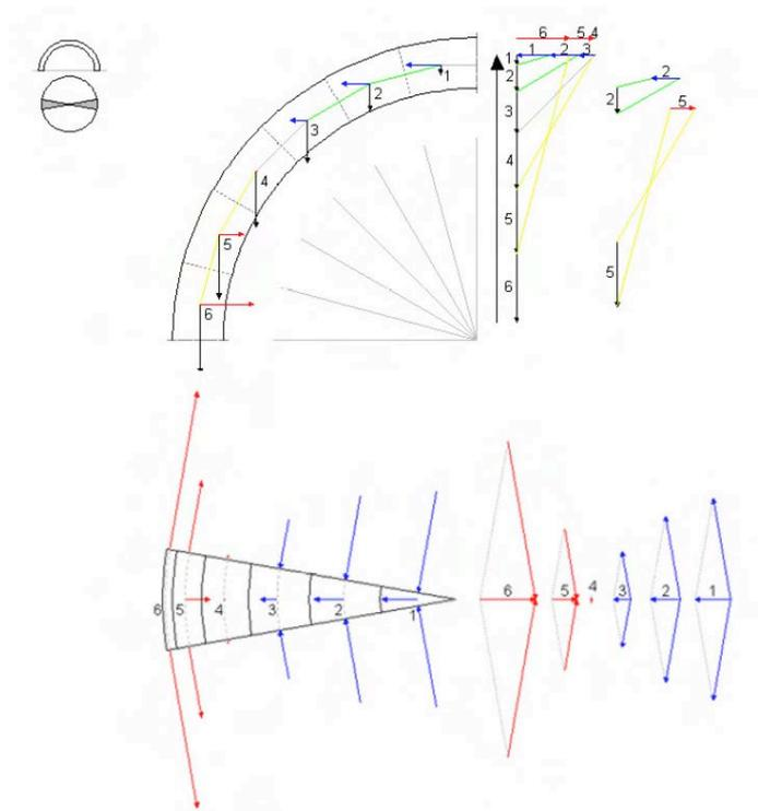
Figure 150: Polygon of forces in a dome section.
