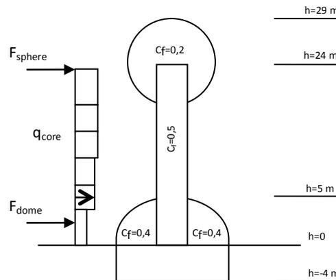
Figure 131: Representative wind pressure forces.
