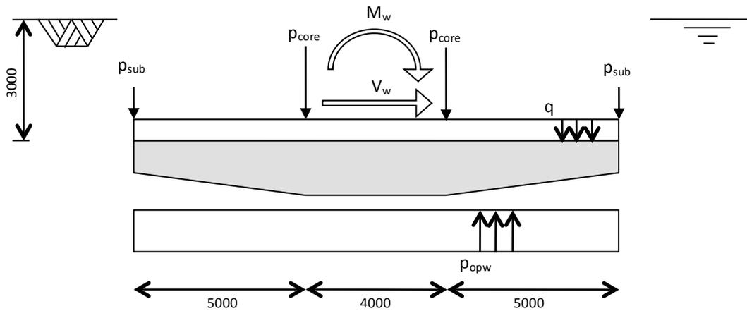
Figure 217: Possible foundation slab with resulting loads of the structure above
