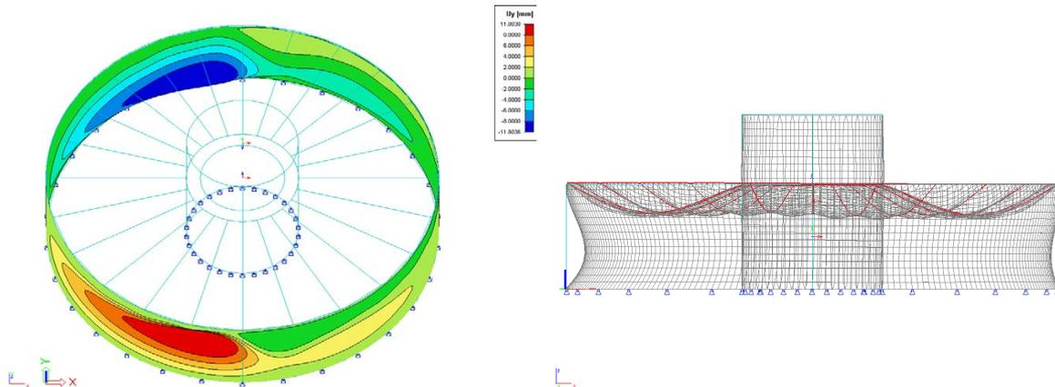
Figure 190: Maximal horizontal deformations in y direction (left) and deformed structure (right)
