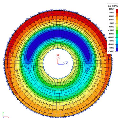
Figure 180: Membrane force nx dome structure for UGT4b
