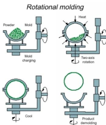
Figure 20: Rotation moulding process
