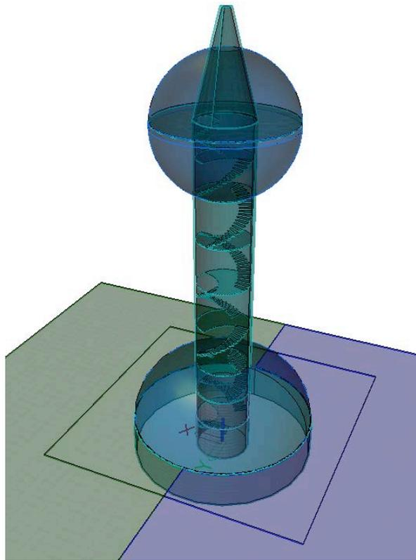
Figure 229: Step 12: The lower dome and removing the building pit.
