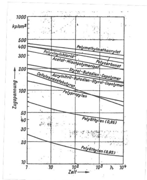
Figure 45: 2% strain limit strength in time for 20 degrees Celsius determined in tensile tests (Gleiter 2002)
