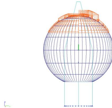
Figure 168: Unevenly distributed snow load in circular zones
