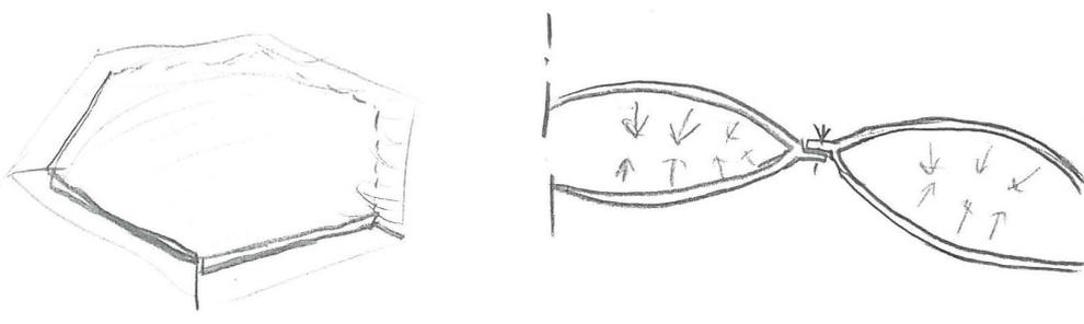
Figure 161: Vacuum formed elements visualised.
