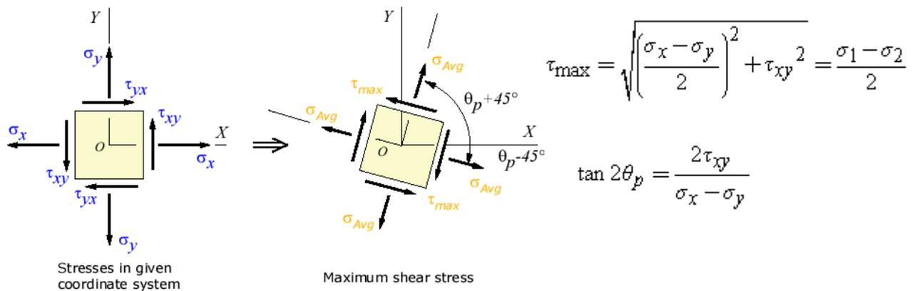
The theory for maximal shear stress assumes that failure will occur when the maximal shear stress reaches a certain value. It is applicable to ductile materials that fail on shear stress rather than tensile stress in a tensile test. The maximal shear stress can be checked with the design value for shear strength. (Hibbeler 2006)
