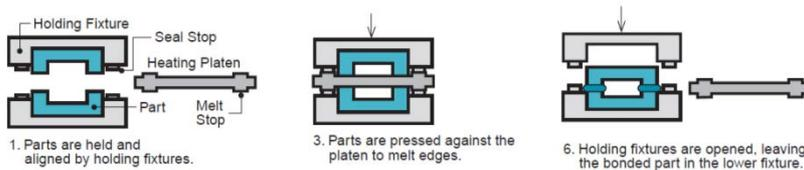
Figure 84: Hot plate welding
