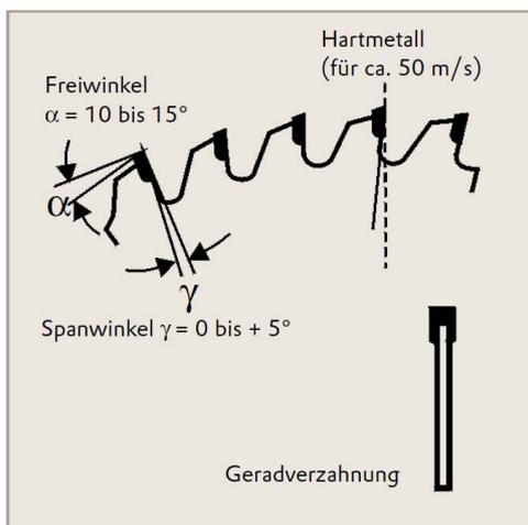
Figure 22: Sawing
