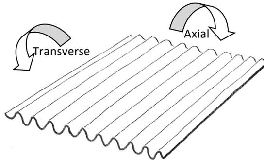
Figure 73: Explanation transverse and axial stiffness
