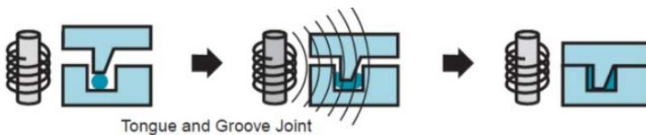
Figure 85: Induction welding
