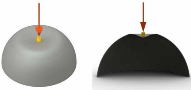
Figure 149: Post buckling behaviour for initial collapse load  $P_0$  (Ameri 2011)
