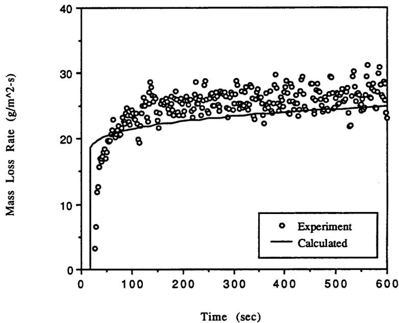
Figure 120: Mass loss rate; experimental data compared to calculated values. (Rhodes 1994)
