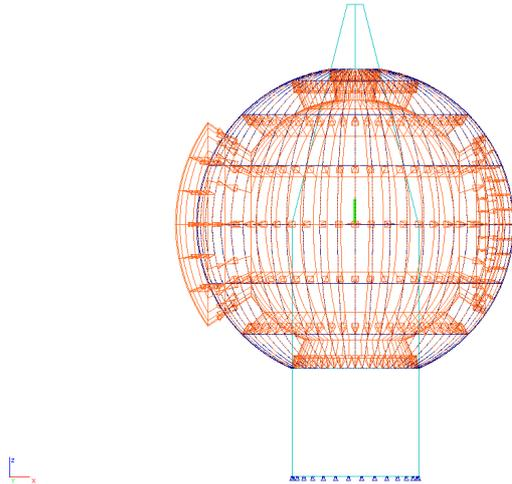
Figure 165: Distribution of wind load in three zones
