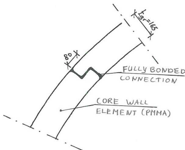
Figure 199: Core elements bonded by polymerizing glue
