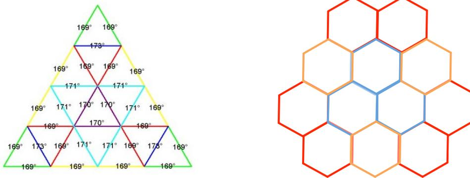
Figure 162: Elements in a 4v dome and its dual
