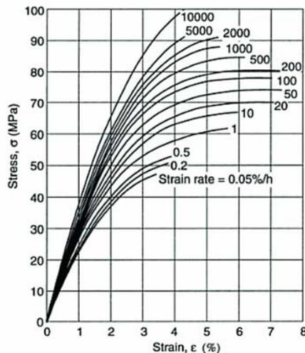
Figure 50: Strain-rate dependence PMMA [polymer processing fundamentals- T. Osswald]
