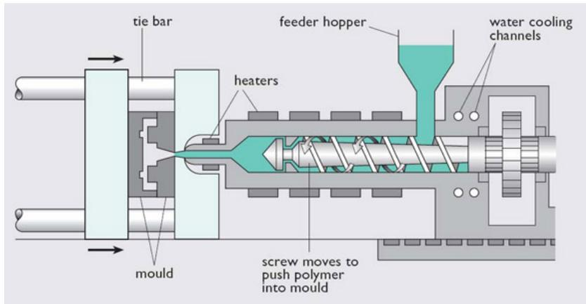
Figure 17: Injection moulding process
