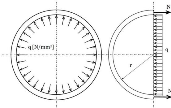
Figure 187: Picturing the ring stresses in a cylinder caused by a uniform compression
