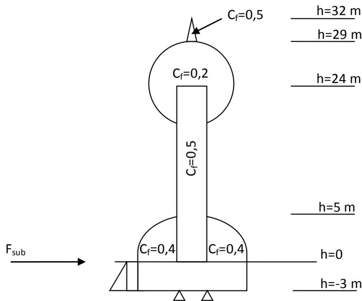
Figure 138: side profile with subsurface load
