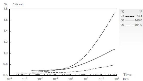
Figure 2: Strain in time for different temperatures PC (at 15 MPa) (GE Plastics 2004)
