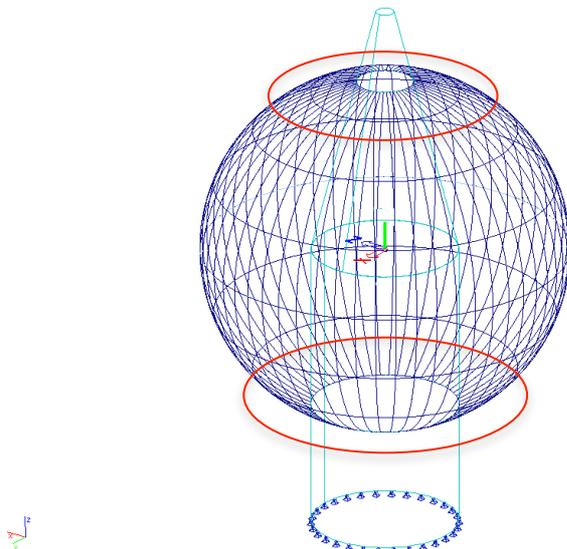
Figure 171: areas with stresses higher than the design stresses
