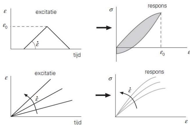
Figure 28: Response of a viscoelastic material to a constant strain rate (Vegt 1991)
