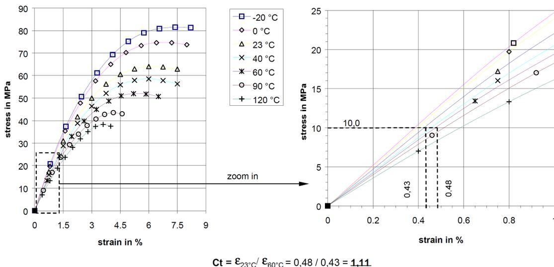
Figure 123: Determination design factors for temperature influence on PC, short term, stable environment. (ETAG010 2002)
