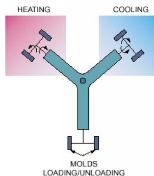
Figure 21: Carousel rotational moulding machine
