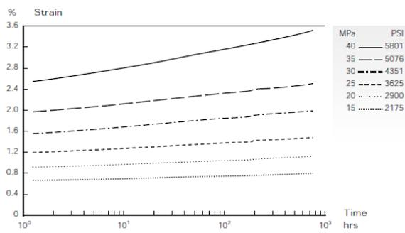
Figure 40: Strain in time for different stresses PC (at 23 °C) (GE Plastics 2004)
