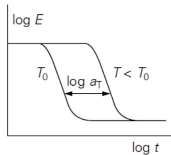
Figure 92: Shifting factor (Vegt 1991)
