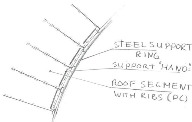
Figure 209: Top view PC roof segments and steel ring, top of the sphere
