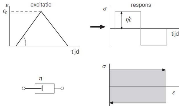
Figure 27: Response of viscous material to a constant strain rate (Vegt 1991)
