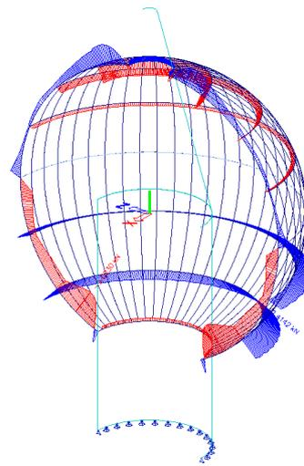
Figure 175: Normal forces in ribs, UGT2. Red for compression, blue for tension
