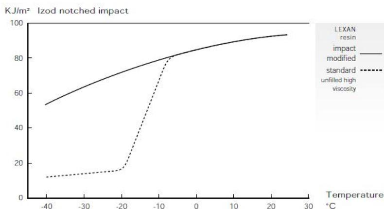
Figure 59: Impact resistance versus temperature (GE Plastics 2004)
