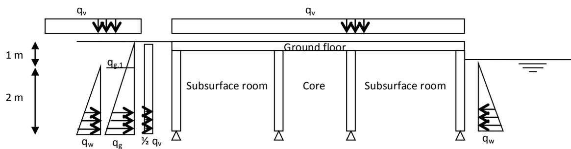
Figure 186: Loads on subsurface room wall
