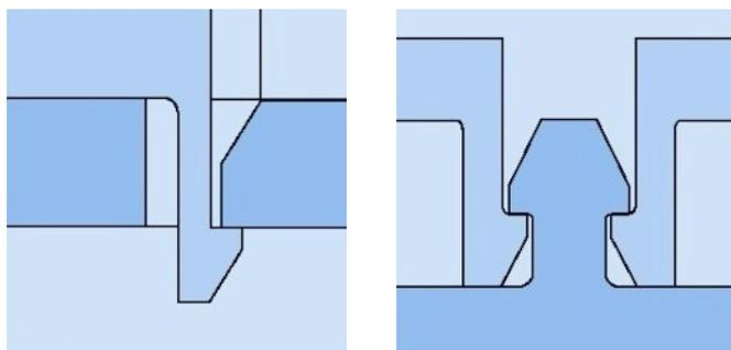
Figure 90: Two possible snap fit joints, a cantilever snap arm and a cylindrical snap fit (MIT 2012)
