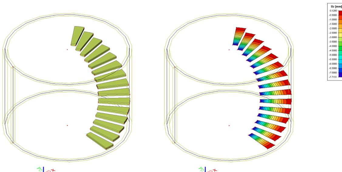
The deformation appears to be indeed less than calculated, a thickness of 80 mm is sufficient, the steps now deflect 7,7 mm. The stresses in the core due to the cantilevering stairs is insignificant, the stress concentrations do not exceed 0,5 MPa.
