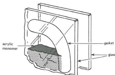
Figure 14: Batch-cell casting
