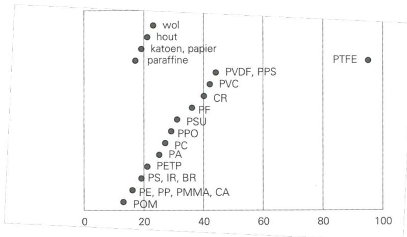
Figure 52: Oxygen index (Vegt 1991)
