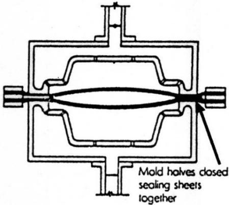
Figure 159: Twin sheet vacuum forming.
