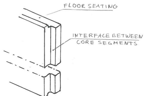
Figure 201: Core element with step joint on two sides
