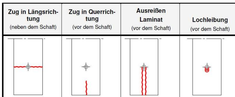
Figure 96: Possible failure mechanisms for a bolted connection (Büv 2010)
