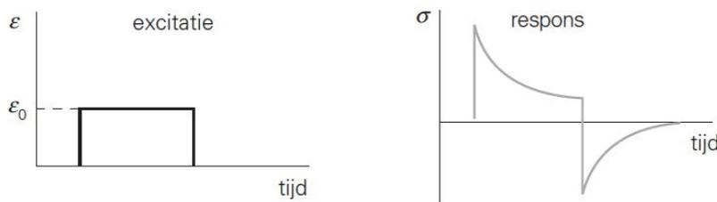
Figure 32: Response of a viscoelastic material to a constant strain (Vegt 1991)
