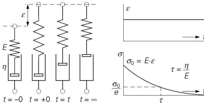
Figure 34: Response of Maxwell model to constant strain – relaxation (Vegt 1991)
