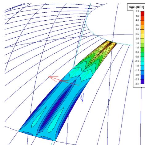
Figure 206: Maximal ring stresses taken by connection
