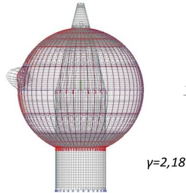
Figure 183: Result of stability calculation for UGT3
