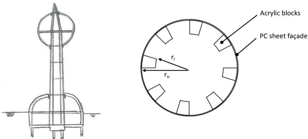
Figure 125: left: Bearing structure with PMMA columns; right: a cross section of the bearing structure (core)
