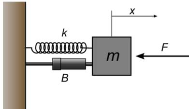
Figure 142: Mass-spring-damper system. (MIT 2012)
