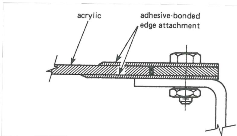
Figure 88: Edge attachment, bonded to acrylic (Stachiw 2003)
