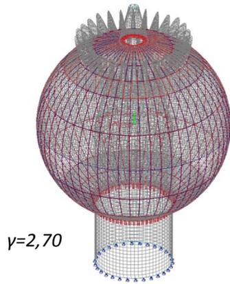
Figure 182: Result of stability calculation for UGT2
