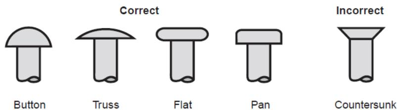
Figure 87: Different fasteners heads (Bayer 2001)
