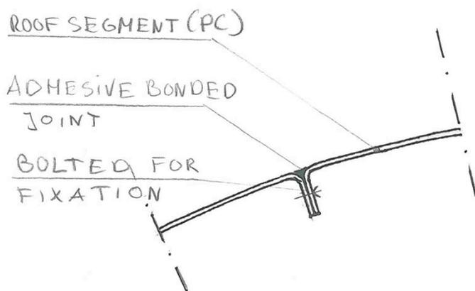
Figure 205: Roof segments connection
