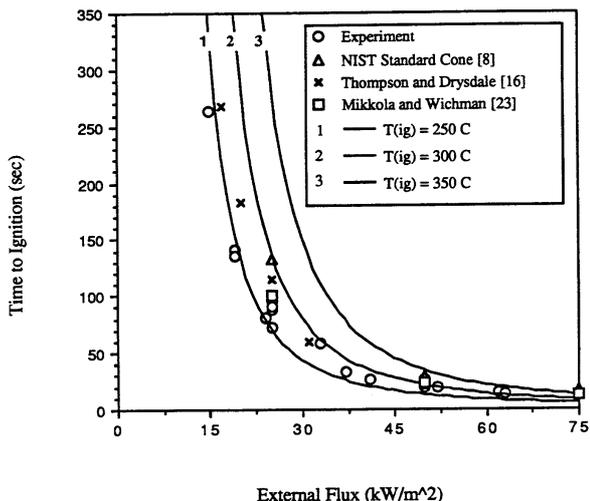
Figure 118: External Heat flux and time to ignition. (Rhodes 1994)
