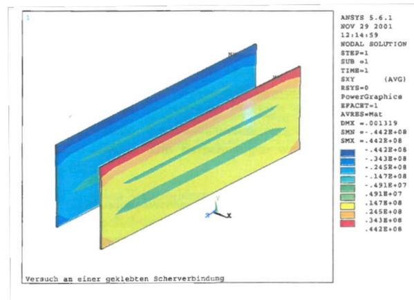
Figure 82: Stress distribution in a glued PMMA samples (Gleiter 2002)
