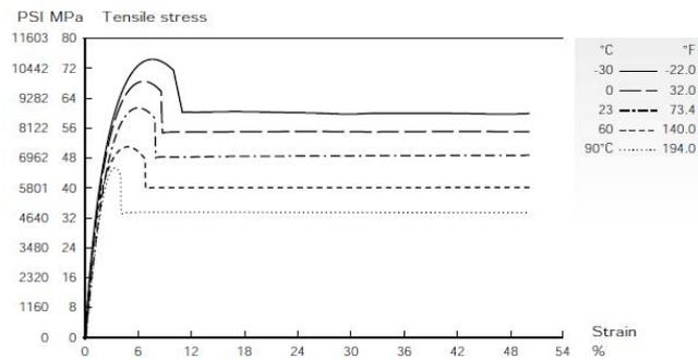
Figure 47: Stress-strain graphs of polycarbonate, Lexan resin 141R (GE Plastics 2004)
