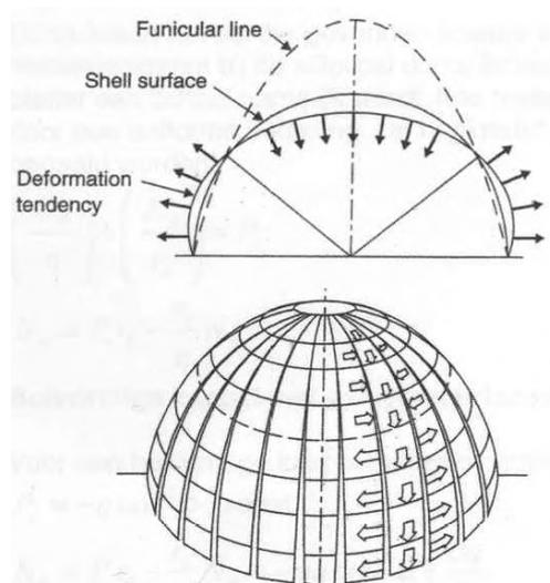
Figure 145: Ring stresses in a dome structure.
