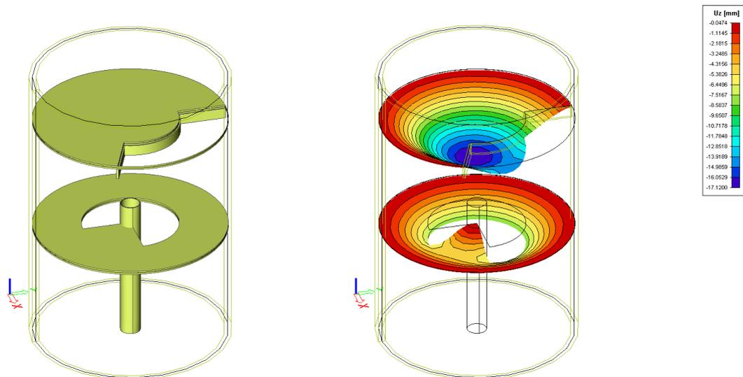
Figure 195: Example of a stairwell for a winding staircase and a spiral staircase, floors of 75 mm
