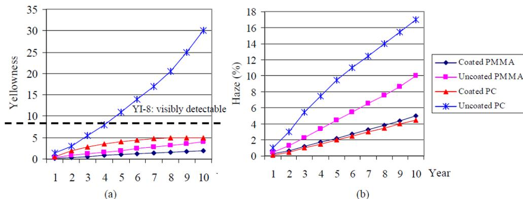
Figure 2.2.1.3 Yellowness Index (a) and Haze of PC and PMMA under UV Exposures
