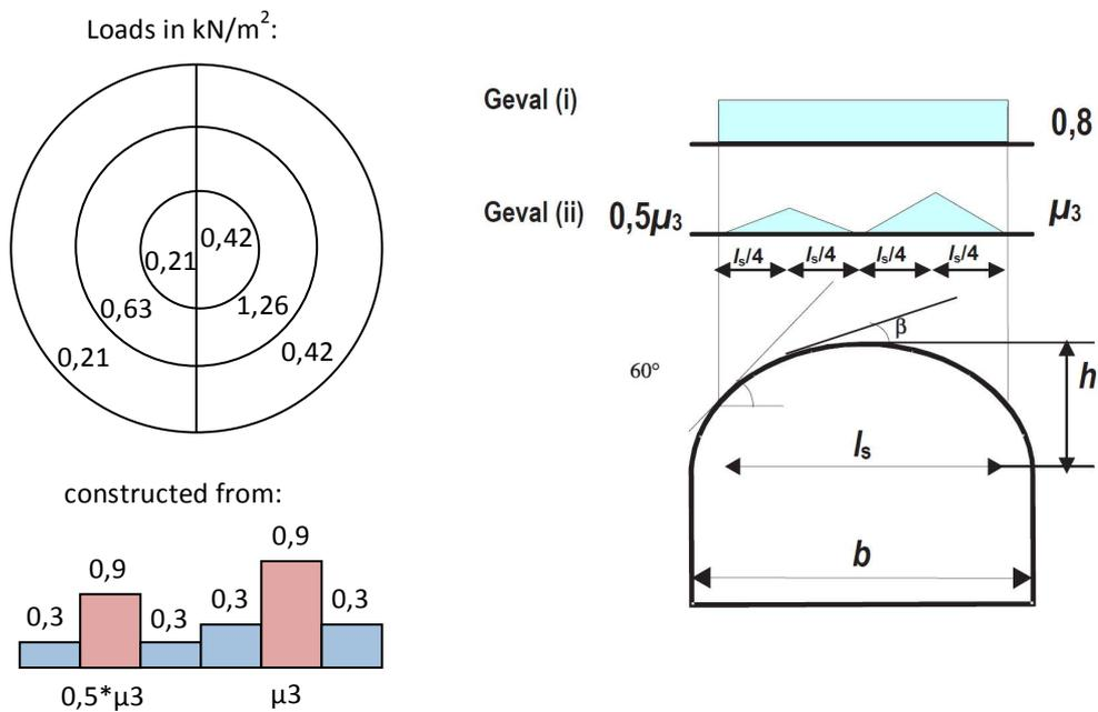
Figure 166: Load zones for asymmetrical snow load. Top view and factors for  $\mu_3$ . (NEN-EN1991-1-3 2003)
