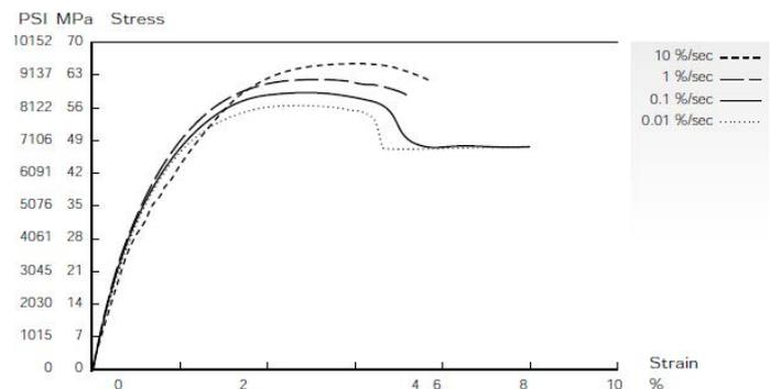
Figure 51: Strain-rate dependence PC (GE Plastics 2004)
