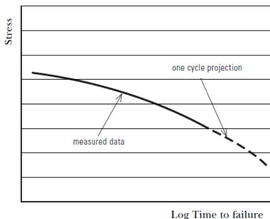
Figure 70: Creep rupture, 1 log (t) extrapolated (GE Plastics 2004)
