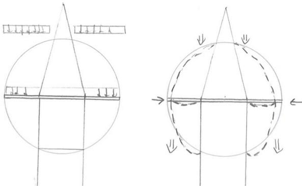
Figure 213: Development of compressive stresses between sphere elements and observatory floor
