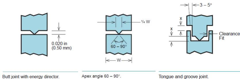
Figure 86: Ultrasonic welding with parts of the same material with energy director tip melting under high frequency vibrations. The molten material creates the bond. (Bayer 2001)
