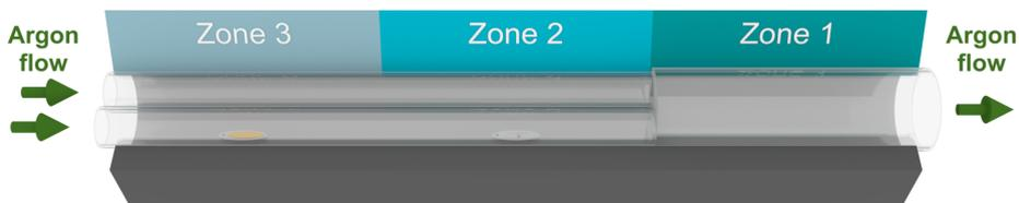
Figure 2.6: Schematic illustration of the three-zone gradient tube furnace from Carbolite Gero. This furnace is connected to an argon gas source at the entrance (at zone 3), and a bubbler system and subsequent exhaust at the back end (at zone 1). For the synthesis of WS<sub>2</sub>, sulfur powder is provided as chalcogen precursor in zone 3, while the substrate and tungsten-based precursor are loaded in zone 2.
