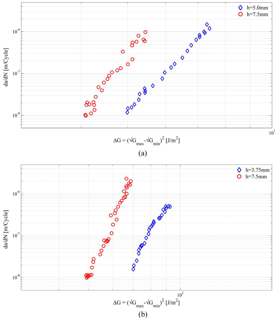
**Fig. 6.** Fatigue delamination with the same crack extension (a)  $a - a_0 = 11.6$  mm for  $h = 5.0$  mm,  $a - a_0 = 12.5$  mm for  $h = 7.5$  mm; (b)  $a - a_0 = 20.9$  mm for  $h = 3.75$  mm,  $a - a_0 = 20.4$  mm for  $h = 7.5$  mm.
