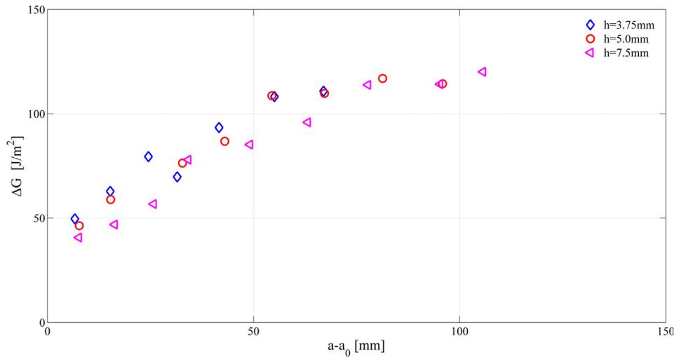
Fig. 3.  $\Delta G$  vs.  $a - a_0$  at a given  $da/dN = 1 \times 10^{-7}$  m/cycle with crack propagation.
