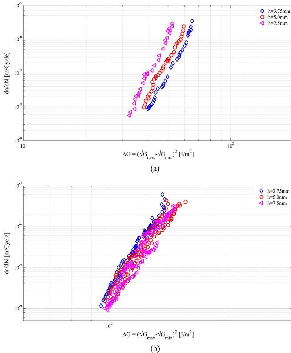
Fig. 5. Fatigue delamination with different amounts of fibre bridging (a) limited fibre bridging; (b) fully developed fibre bridging.
