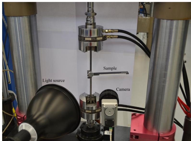
Fig. 1. Fatigue experimental set-up.
