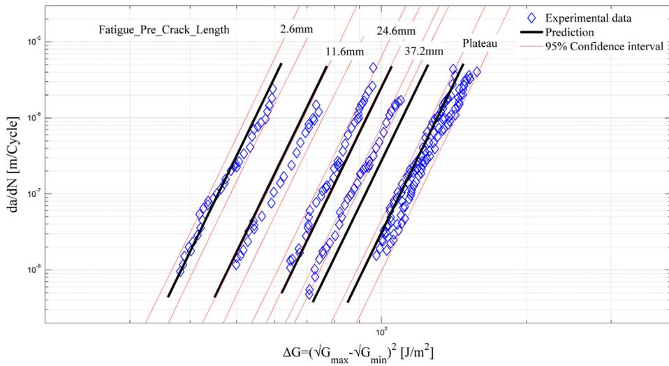
Fig. 10. Fatigue delamination predictions of specimen Sp<sub>32</sub> ( $h = 5.0$  mm).
