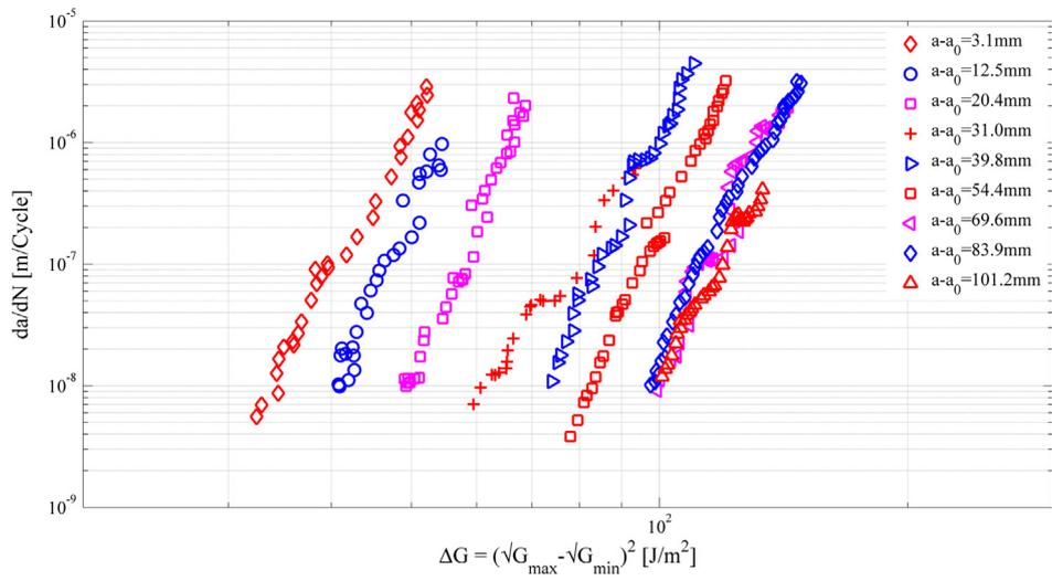
Fig. 2. Fatigue data interpretation with the Paris relation (a)  $h = 3.75$  mm; (b)  $h = 5.0$  mm; (c)  $h = 7.5$  mm.
