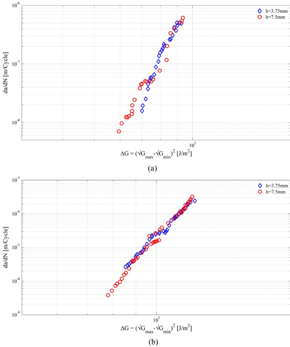
Fig. 9. Fatigue delamination with the same magnitude of  $(a - a_0)/L_{pz}$  (a)  $(a - a_0)/L_{pz} = 0.45$ ; (b)  $(a - a_0)/L_{pz} = 0.78$ .
