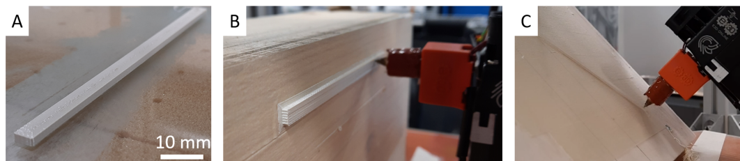
Figure 6.1: LCP tensile specimens printed under different orientations. A: Flat on heated bed. B: Vertically against a wall. C: Diagonally against an incline.
