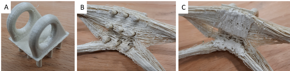
Figure 6.5: Printing and fastening process of the upper lugs. A: Upper lugs as they came out of the printer. B: Pins inserted through nine holes that were made with a soldering iron. C: Pin heads flattened out and integrated with the bracket.
