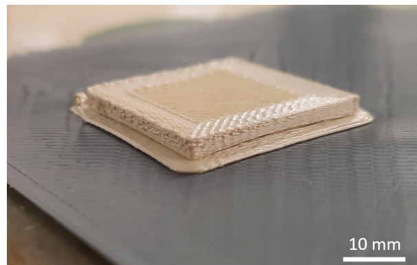
Figure 5.2: Test print of LCP on PLA. Small warpage of the PLA is visible. Releasing the LCP square was no problem
