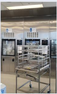
After ultrasonic cleaning the dirty Devices come out of the products move into the washing machines. These machines have different programs and specific devices will also be cleaned chemically. Furthermore, great care will be taken to make sure that products do not touch each other, since that will hinder proper cleaning.
