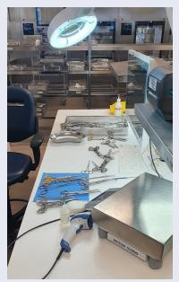
In the clean room the products get checked for cleanliness and function. Then they are weighed to check whether all products are on the net. After this they will be packaged in 'blue medical wrap' and moved to the autoclave.
