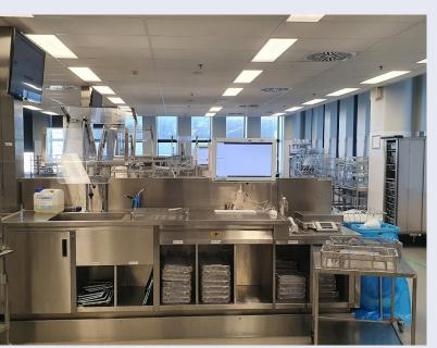
Dirty devices arrive in metal nets by which they will be tracked. Here they will be pre-cleaned by hand and put in the ultrasonic cleaner if the particular devices are compatible with the ultrasonic cleaner.
