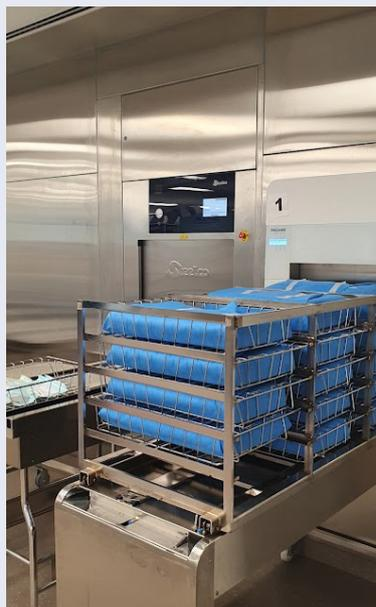
*Here the nets come out in the sterile part. The CSD employees will check whether devices have come out fully dry and check whether the autoclave program has run appropriately.*
