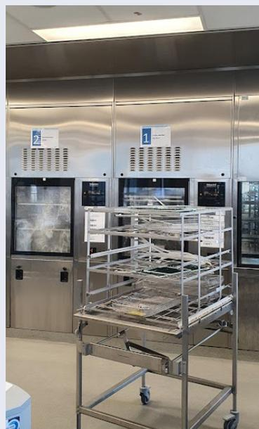
*After ultrasonic cleaning the dirty products move into the washing machines. These machines have different programs and specific devices will also be cleaned chemically. Furthermore, great care will be taken to make sure that products do not touch each other, since that will hinder proper cleaning.*
