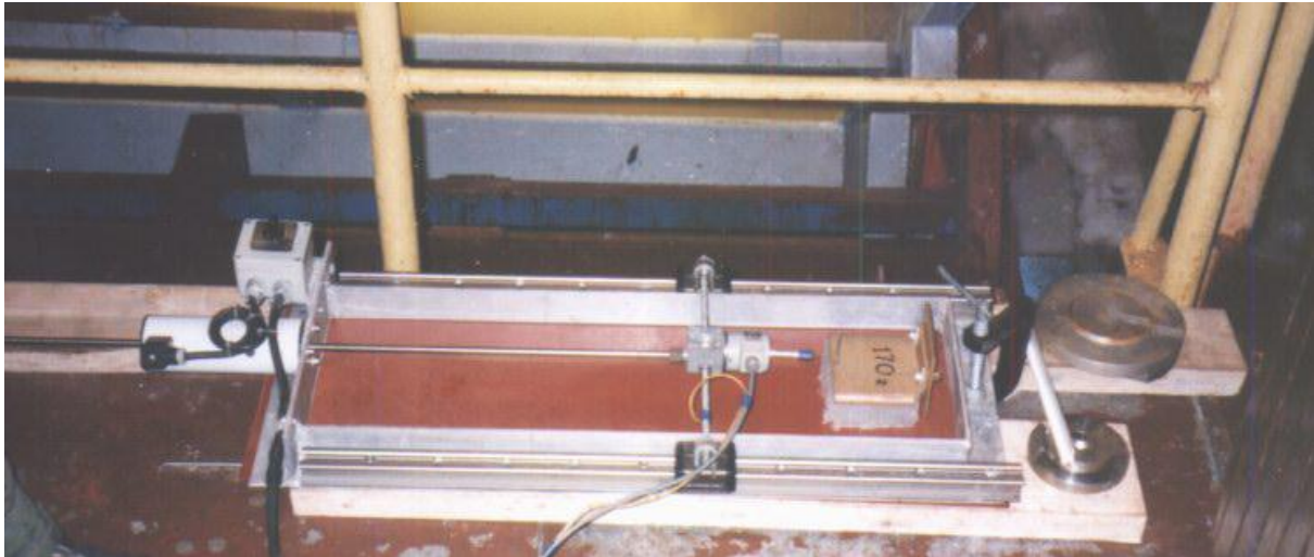
Figure A-7: Measuring the dynamic friction factor
