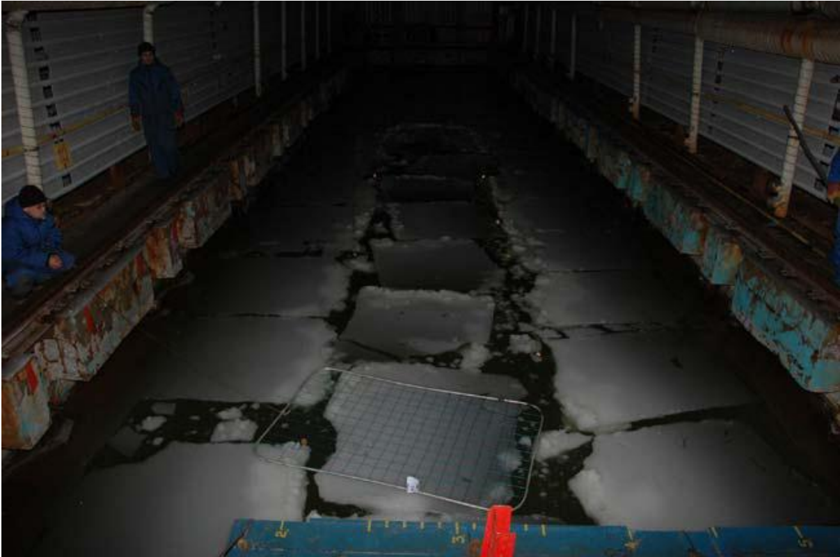
Figure A-4: Broken ice with dimensions of 100 m x 100 m and a concentration of 8/10.
