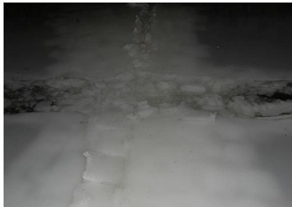
Figure 2-20: The keel of the hummock can be seen through the consolidated layer.
