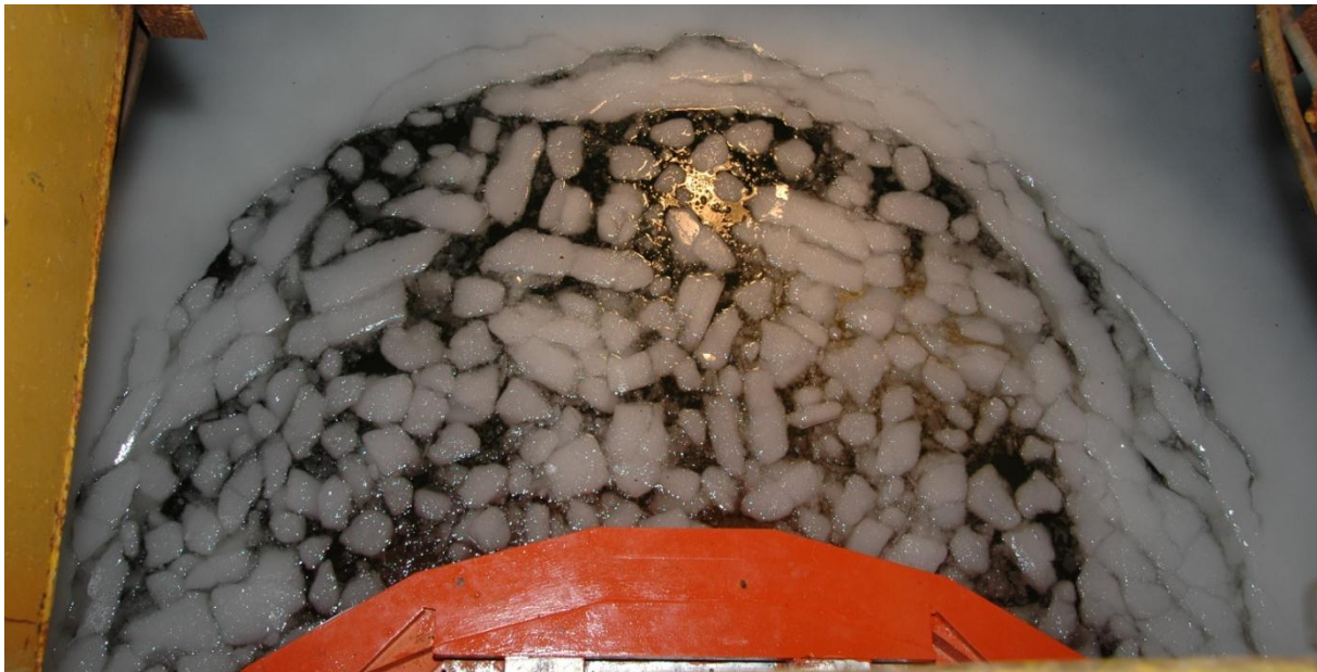
Figure 3-22: Size of the failed ice. The picture was taken after test 3-1: 1.5 m thick ice at 0.5 m/s and a zero degree trim angle.
