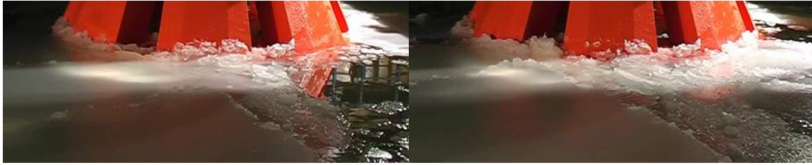
Figure 2-10: 1m thick 100 m broken ice at 0.75 m/s. Time lapse series clearly showing rafting. Time interval is 152 s.
