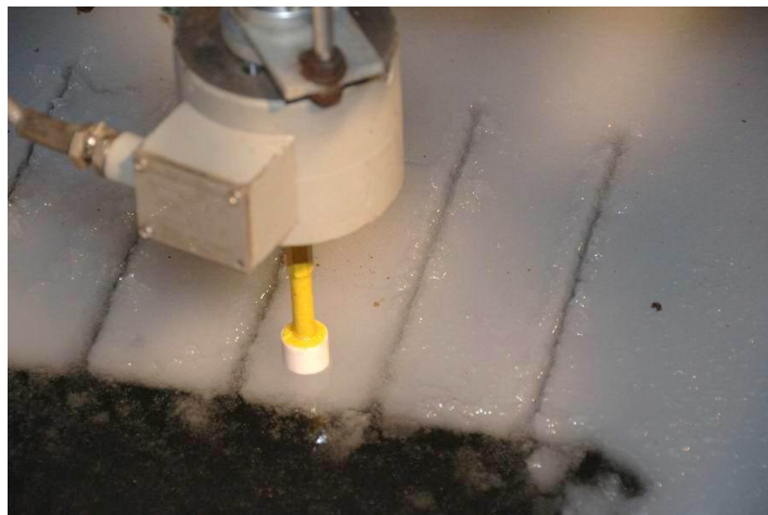
Figure A-6: Ice bending strength measurements being performed
