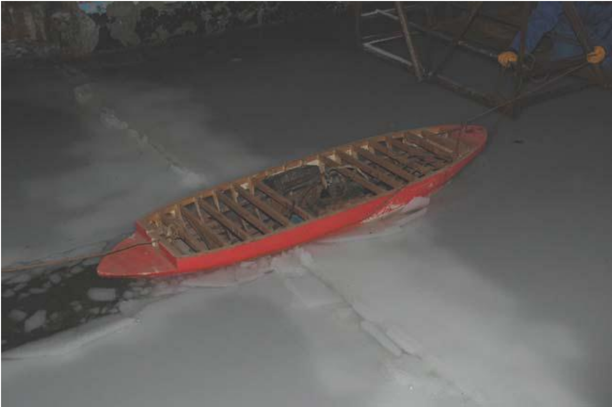
Figure A-5: A channel being created in a hummock using an icebreaker model.
