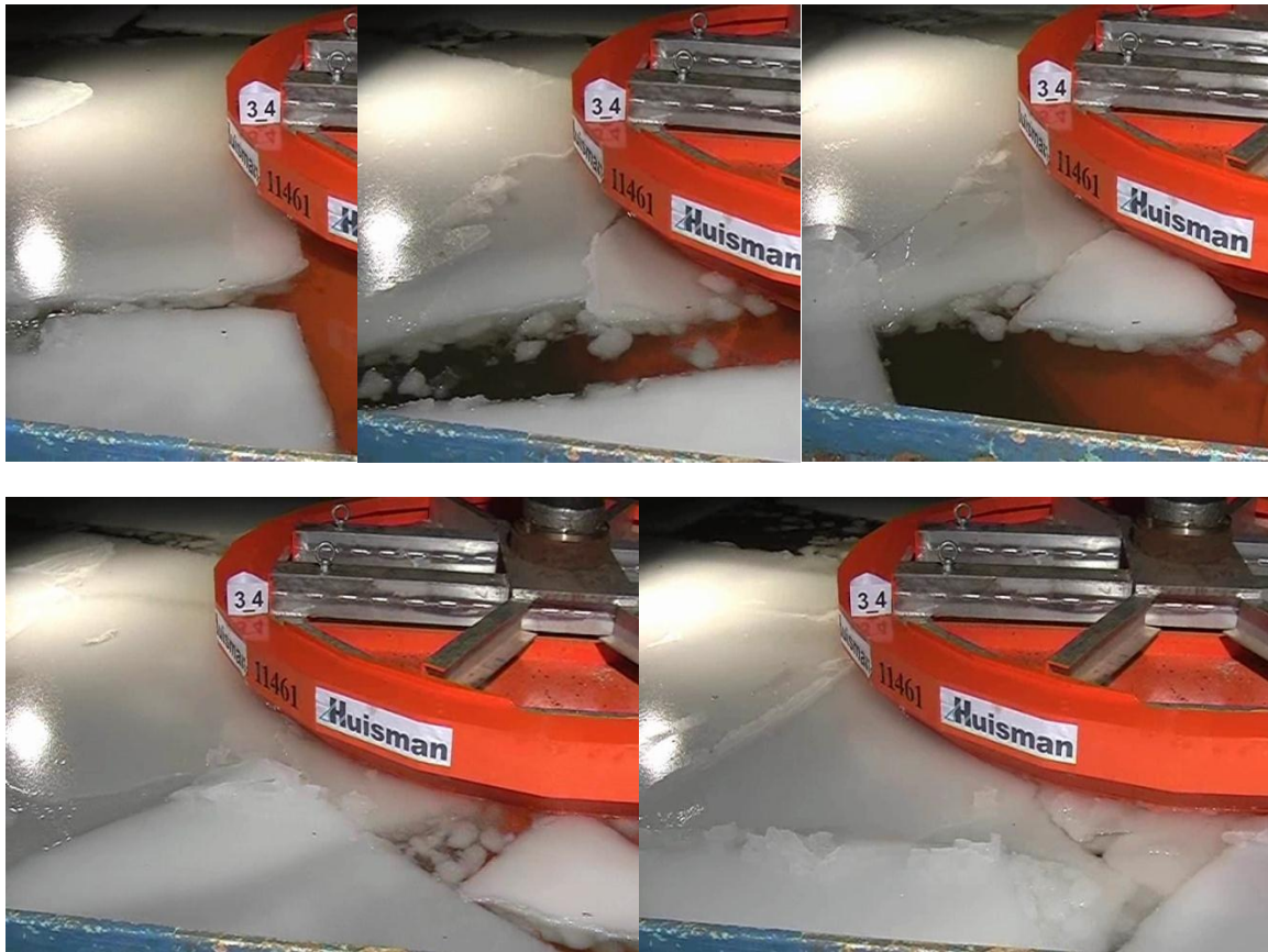
Figure 2-17: 1.5m thick 100 broken ice. Time lapse series showing rafting and buildup of ice. Time interval is 114 s.
