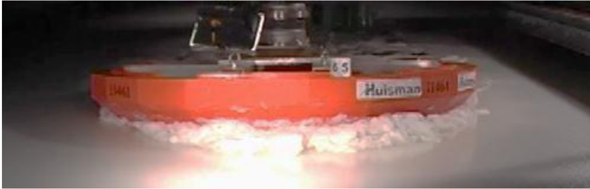
Figure 2-35: 3.0 m thick ice at 5.0 trim angle. Note that there is more rubble.
