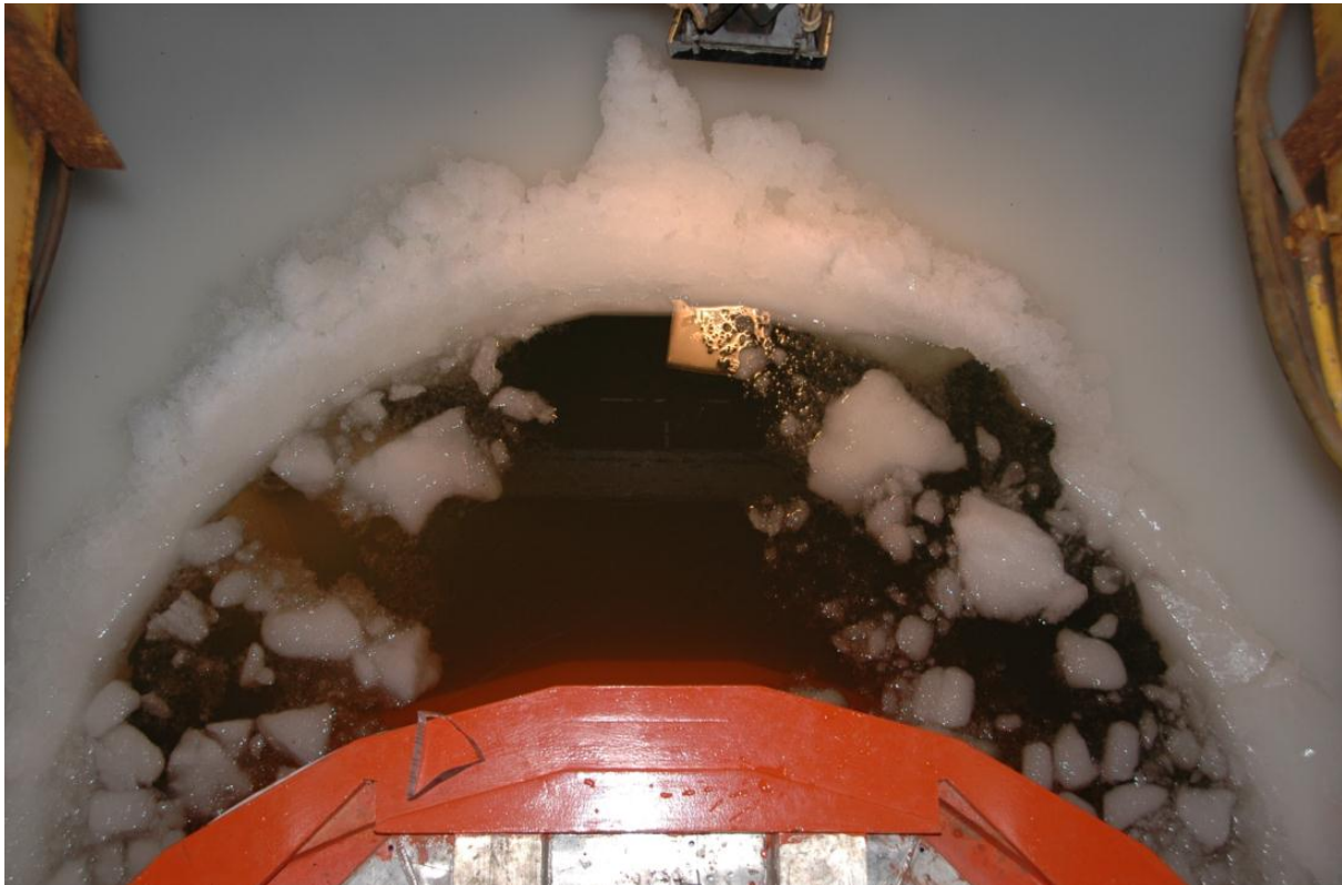
Figure 2-36: The vessel-ice interface clearly shows that crushing took place after the model had been pulled back.
