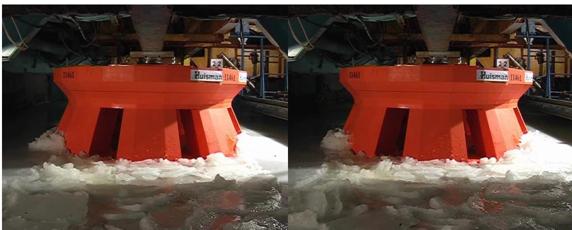
Figure 2-8: Both pictures show 2m thick with a 80m wide channel moving at 0.75 m/s: Notice the rubble is slightly more mobile over time then in 40 m wide channel.
