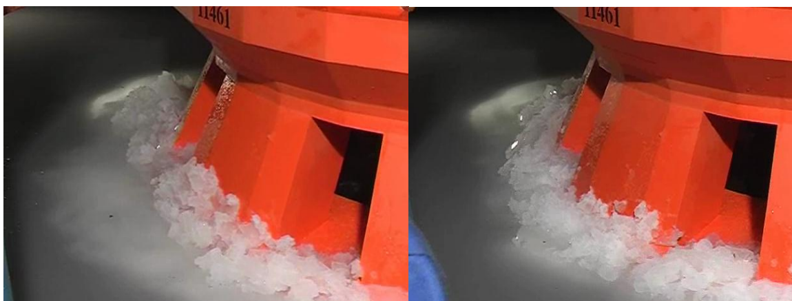
Figure 2-5: 1m thick level ice. Left: 0.75 m/s. Right: 1.50 m/s. Notice the difference in extent of the submerged ice.
