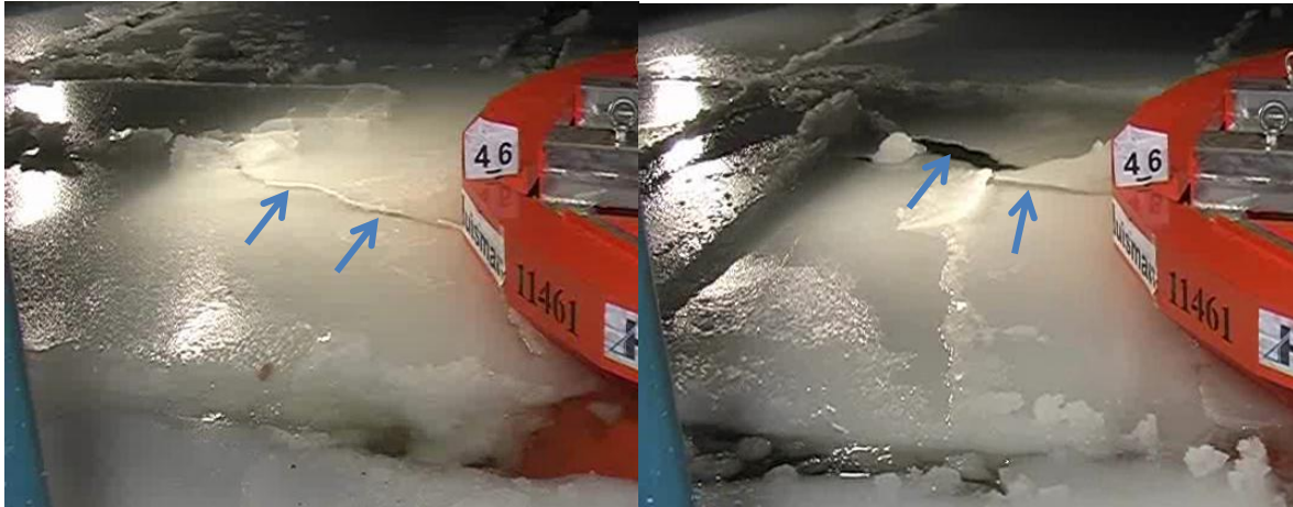
Figure 2-18: 100m broken ice. The arrows show the radial crack which split the ice floe.
