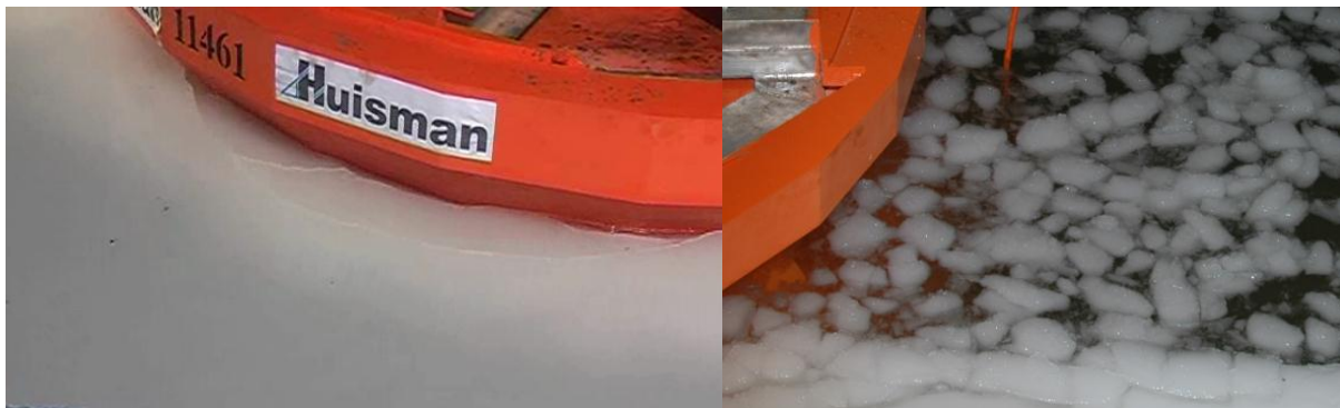
Figure 2-25: Left: Circumferential crack extend further outwards. Right: the resulting ice pieces are slightly larger.
