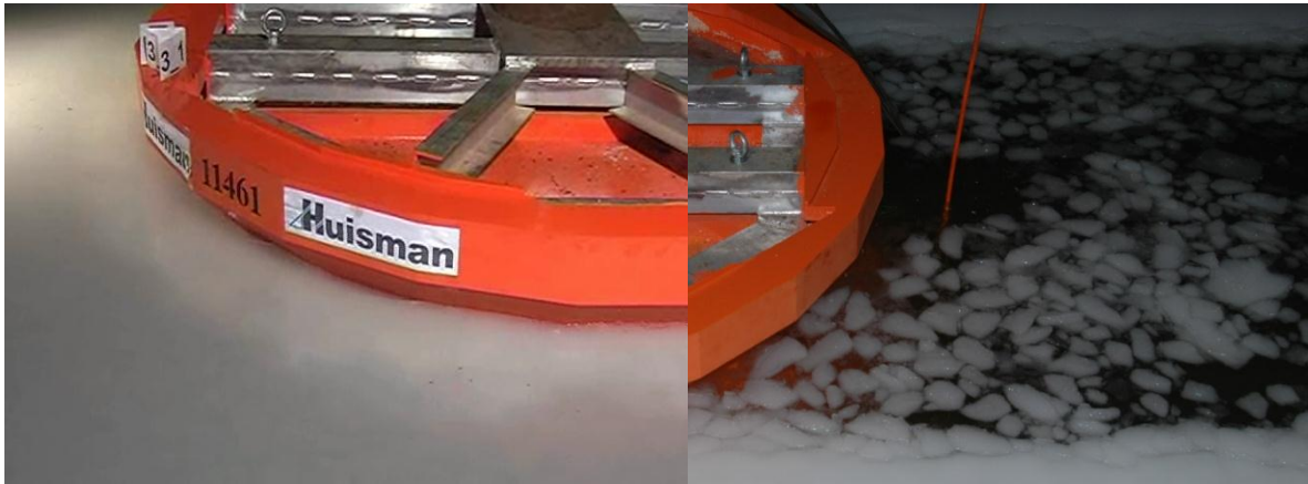
Figure 2-28: 0.5 m/s ice velocity. The base case.
