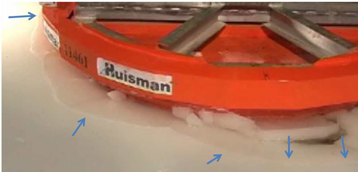
Figure 2-26: The largest circumferential crack observed in the test footage, extending over 150° of the vessel.
