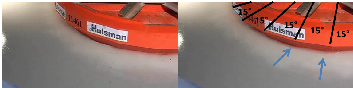
Figure 2-23: Left: normal situation. Right: one of the larger visible circumferential cracks. When estimating the ice action size it is easy to compare them to the hull of the vessel since it is not fully circular but rather 24-sided polygon, resulting in flat planes 15° apart.
