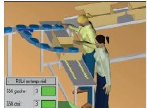
Figure 5a, 5b and 5c: a: The digital CAD model with digital human model. b: Evaluation of field of view by different point of views. c: Continuous RULA evaluation of gesture simulation.
