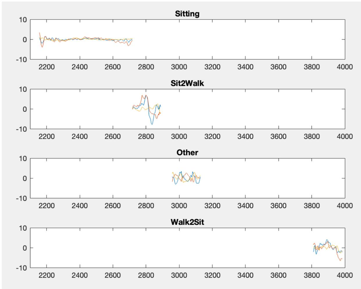
Figure 12: Plot of data extracted from the IMU accelerometer corresponding to each activity.
