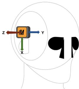
Figure 1: IMU placement and axis direction
