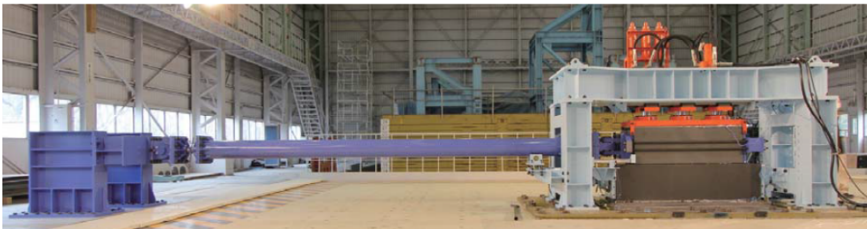
Figure 6.3: Large Scale Earthquake Simulator experiments at the National Institute for Earth Sciences Research and Disaster Resilience, Japan (Collaboration NAM & UU). Taken from (Fukuyama et al. 2014)
