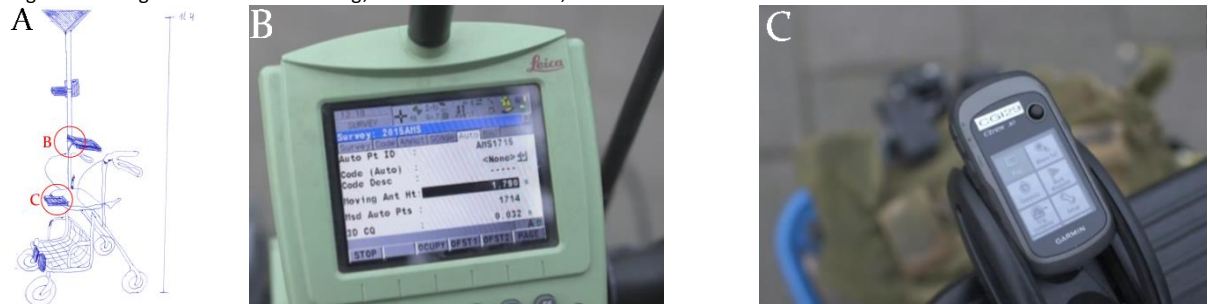
Figure 6: Image A shows the setting, B shows a RTK GPS, and C shows a handheld GPS
