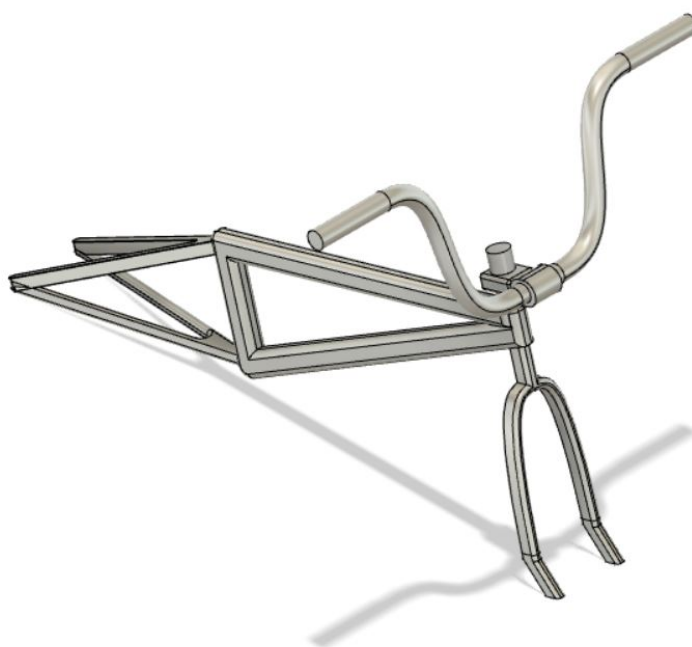
Figure D.1: CAD model of the BMX bicycle frame created using Autodesk Fusion 360.
