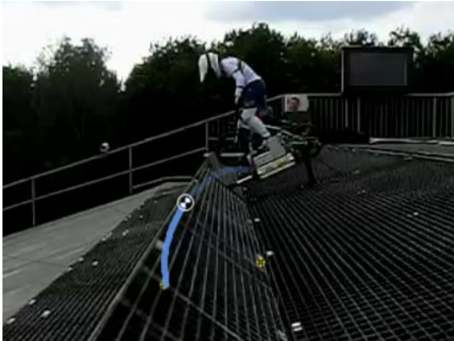
Figure 3.12: The tracking of the gate in Kinovea. The blue line shows the time history of the point being tracked. Due to practical reasons the tracking was done in reverse.
