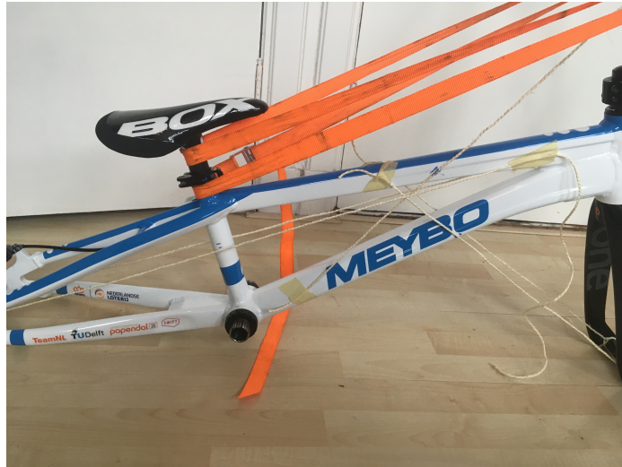
Figure 3.5: The center of mass of the BMX SX frame. The three ropes cross at approximately the same location.
