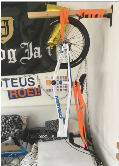
Figure 3.6: The experimental setup to determine the oscillation time of the frame. The rear wheel is used as the rotation point. The orange lashing strap is used to fixate the steering assembly. The right figure shows an exaggerate overview of the pendulum motion of the bicycle. As seen, the center of mass will swing in a perfect circle.
