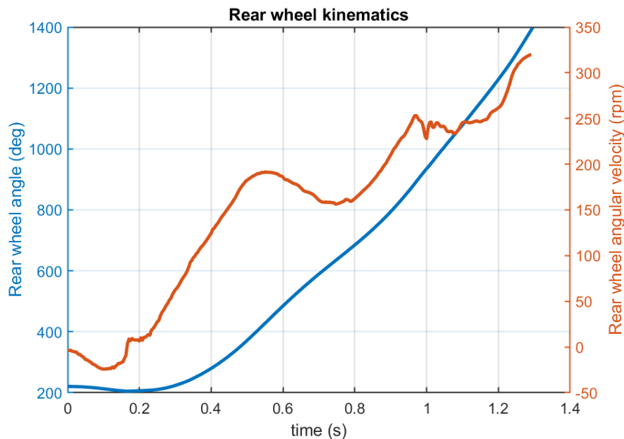
Figure 3.18: Kinematics of the rear wheel as a function of time. The blue line is the rotation of the rear wheel and the orange line shows the angular velocity of the rear wheel expressed in revolutions per minute (rpm). At approximately 0.17 seconds there is a huge jump visible in the angular velocity, indicating that the wheel is slipping. Data taken from Melle van Dilgt [11].
