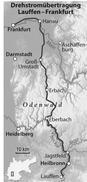
Figure 140: AC transmission between Lauffen and Frankfurt (1891)
