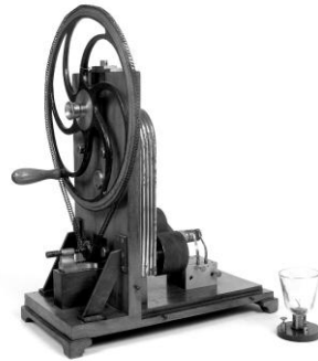
Figure 63: Clarke’s dynamo with the rotating magnets and the commutator (1835)
