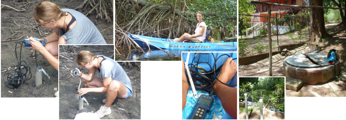
Figure A.2: Manual measurements in the floodplain piezometers, EC and water level (left top and bottom figures). Manual measurements in the estuary with the kayak (middle top and bottom figures). And well W_3 , together with the already existing piezometers in the alluvial aquifer (right figures).
