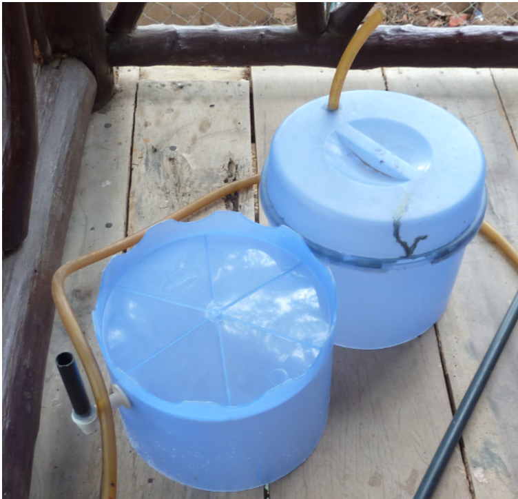
Figure A.3: Self-made seepage meters
