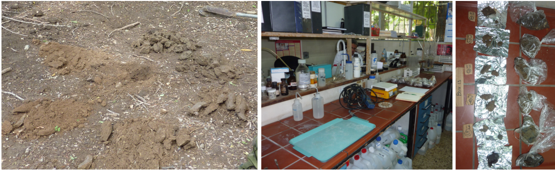
Figure A.6: Retrieving soil samples by digging holes with an auger (left figure), then analyzing them in the lab of CIRA (middle figure), with the sequence of samples for one location depicted in the right figure.
