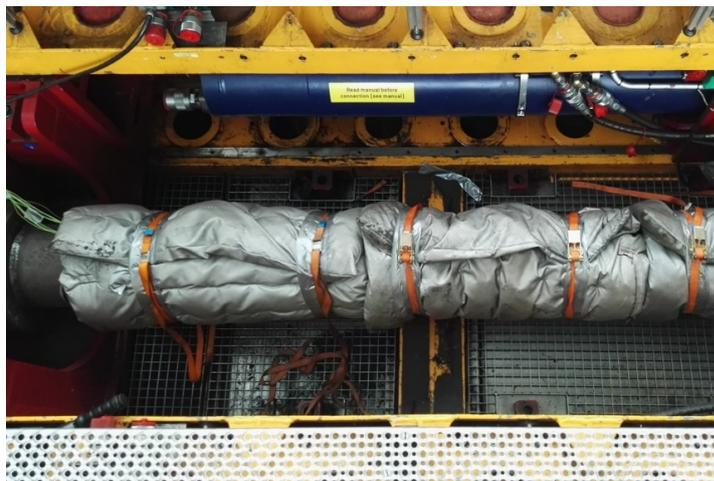
Figure 6.13: Liner for the thermal test installed in the RETF and insulated with thick (gray) blankets to prevent any heat losses.
