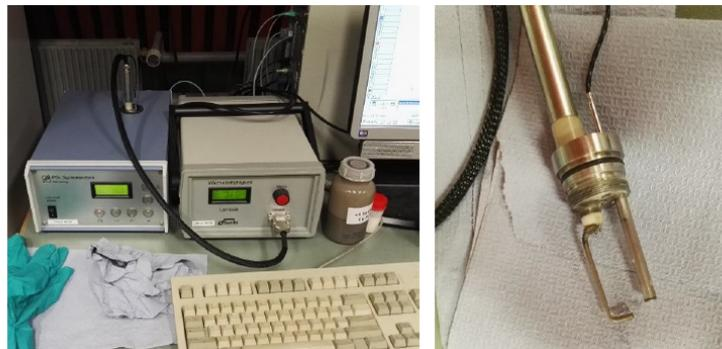
Figure B.1: Setup for the measurement of the thermal conductivity of liquids using the hot wire method. The picture on the right shows the wire and temperature sensor. These are inserted to the device shown in the left picture which controls the ambient temperature and conducts the measurements.
