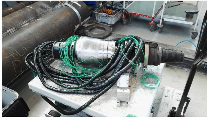
Figure 6.11: Cone for the thermal test with 30 thermocouples and corresponding wiring installed. The wires leave the rear of the cone in two cable batches will be connected to the data acquisition computer.
