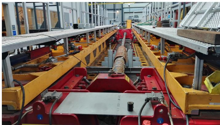
Figure 6.1: RETF (Rotary Expandable Test Facility) in the Shell laboratory in Rijswijk with 9 5/8" liner installed for the split cone test.
