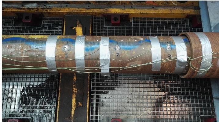
Figure 6.3: Placement of thermocouples on the outside of the single liner section for the split cone test. The thermocouples are welded to the liner at locations 1, 2 and 3 as marked on the liner. Before welding the surface is first cleaned to ensure good contact.
