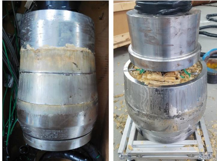
Figure 6.6: Left, the split cone after the test. It can be seen how the lubricant film is broken at the cuts of the split segments. On the right, the top segment has been removed to show that the gap has filled up with lubricant during the expansion.
