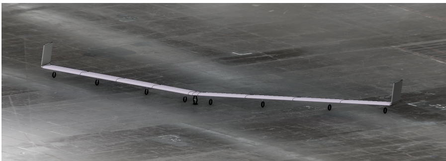
Figure 6.22: All sections connected, including the wingtips.
