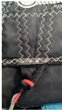
Figure 4.20: A photograph presenting the way the harness attachment cable is attached to the structure.
