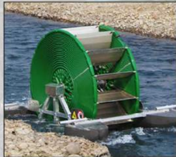
Water powered system to pull water from primary to secondary waterways
