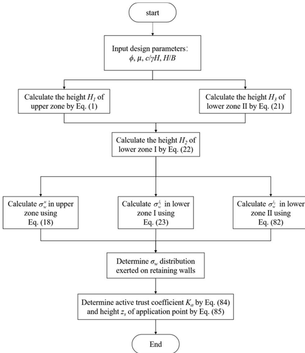
Fig. 6. Calculation flowchart.
