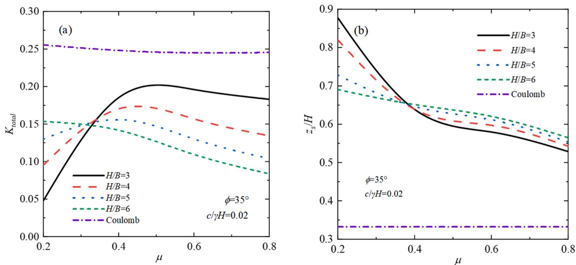
Fig. 15. Effect of wall-soil interface roughness factor under various aspect ratios on: (a) active thrust coefficient and (b) normalized height of application point of active thrust to wall base.
