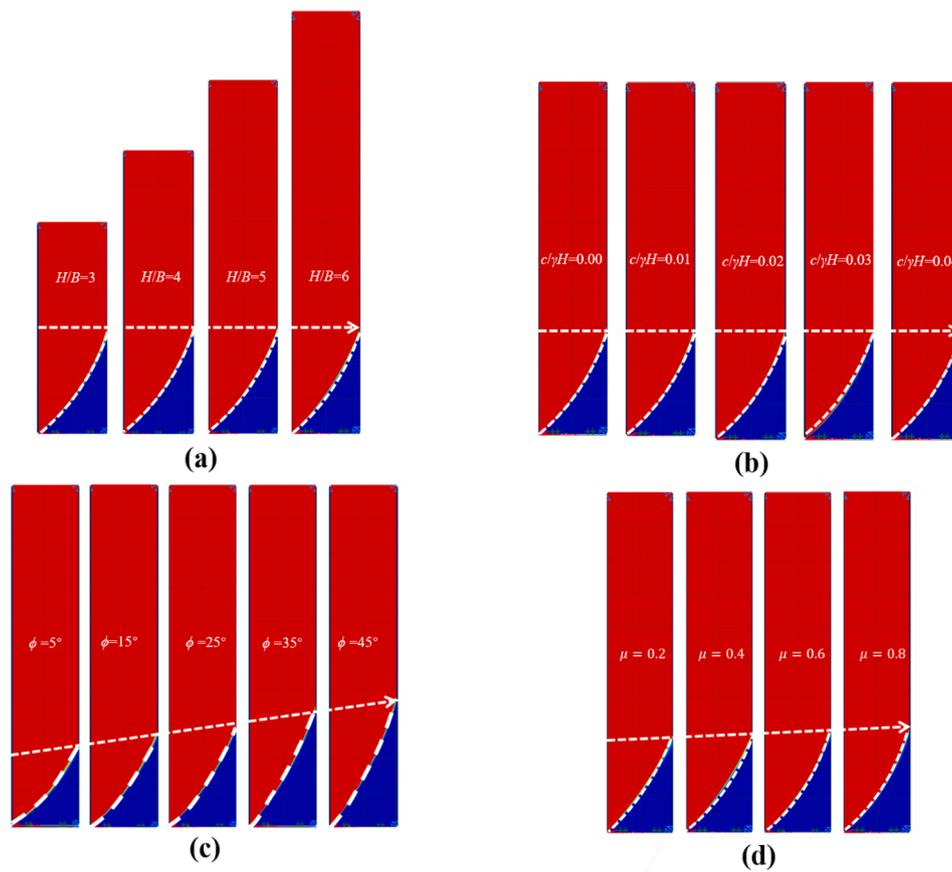
**Fig. 3.** Effect of four dimensionless parameters on the failure mode of narrow soils behind rotating wall about the top: (a) aspect ratio ( $c/\gamma H = 0.027$ ,  $\phi = 25^\circ$  and  $\mu = 0.6$ ); (b) soil cohesion ( $H/B = 0.2$ ,  $c/\gamma H = 0.027$  and  $\mu = 0.6$ ); (c) soil friction angle ( $H/B = 0.2$ ,  $c/\gamma H = 0.027$  and  $\phi = 25^\circ$ ) and (d) roughness factor ( $H/B = 0.2$ ,  $\phi = 35^\circ$  and  $\mu = 0.6$ ).
