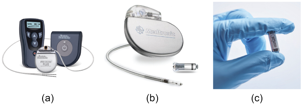
Figure 1.1.: Examples of implantable medical devices available on the market, also showing the trend of miniaturisation of these devices. (a) Spinal cord stimulator from Boston Scientific [4]. (b) One of the world's smallest pacemakers from Medtronic, compared to its predecessor [5]. (c) Inductively powered vagus nerve stimulator from SetPoint Medical [6].
