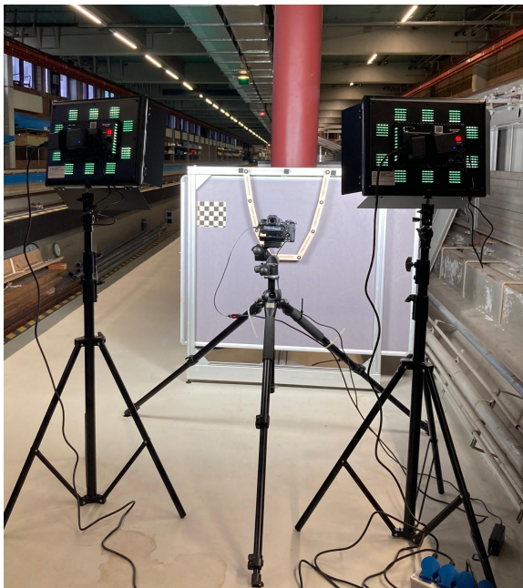
(a) An image of the front of experimental setup. A camera and two LED lights are placed in front of the framework. The camera detects the motion of the model dropper and the checkerboard connected to the framework is used for calibrating the camera.
