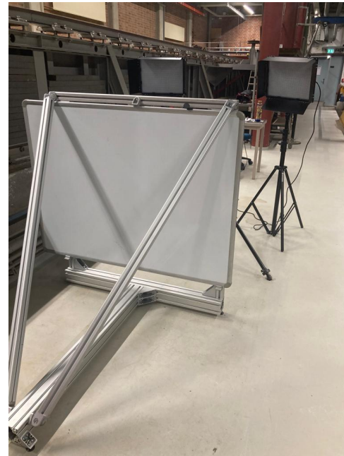
(b) An image of the back of the experimental setup. A framework of item profiles is constructed in order to attach the model dropper to. The framework has a T-profile as basis in order to decrease the number of parts that need to be leveled.
