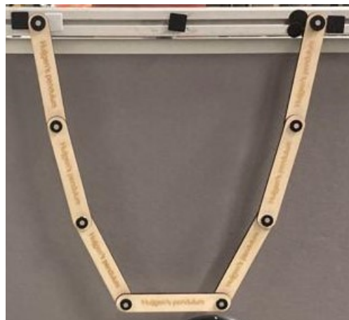
Figure 7.3: The model dropper in the experimental setup. The two outer pendulums are placed 0.4 metres apart. Each node on the mussel dropper has a circle attached to it which is used to determine the positions later on.
